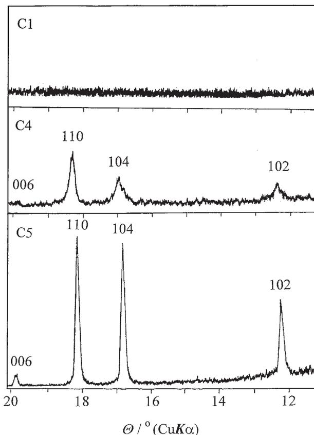
Figure 2. Characteristic parts of X-ray powder diffraction patterns of amorphous chromium hydroxide (sample C1) and its thermal decomposition products (samples C4 and C5). Diffraction patterns were recorded at room temperature.
