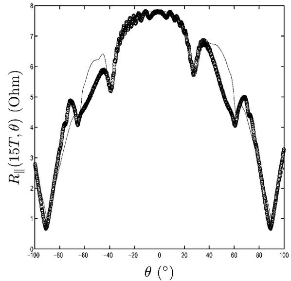
FIG. 3. The angular dependent magnetoresistance is shown for current parallel to the  $a$ - $c$  plane at  $T = 1.4$  K,  $B = 15$  T. The open circles belong to the experimental data, and the solid line is our fit based on Eq. (7).
