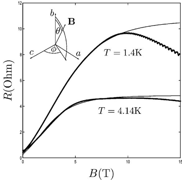
FIG. 1. The magnetoresistance is plotted for  $T = 1.4$  and  $4.14$  K as a function of magnetic field. The thick solid line is the experimental data, and the thin one denotes our fit based on Eq. (7). The inset shows the geometrical configuration of the magnetic field with respect to the conducting plane.
