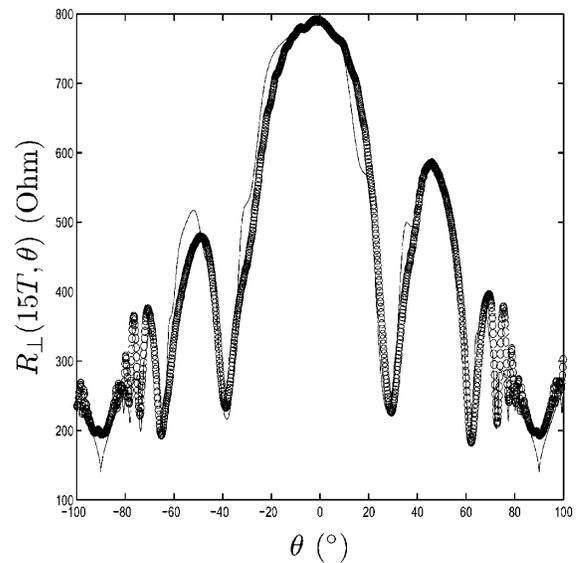
FIG. 4. The angular dependent magnetoresistance is shown for current perpendicular to the  $a$ - $c$  plane at  $T = 1.4$  K,  $B = 15$  T. The open circles belong to the experimental data, and the solid line is our fit from Eq. (7).
