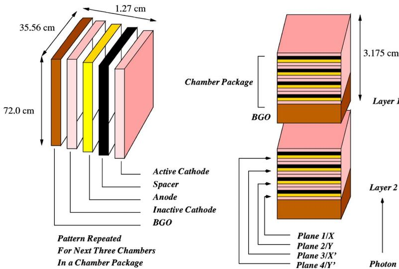
FIG. 5. (Color online) Schematic of NMS chamber package.
