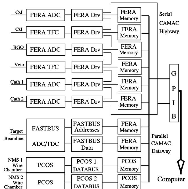
FIG. 6. Data flow diagram for the experiment.
