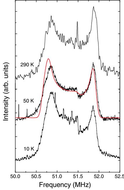
FIG. 1 (color online). Frequency swept  $^{75}\text{As}$  NMR powder spectra of  $\text{LaFeAsO}_{0.9}\text{F}_{0.1}$  measured at  $H_0 = 7.0494$  T. The thick solid red line is a simulation of the powder spectrum as described in the text.
