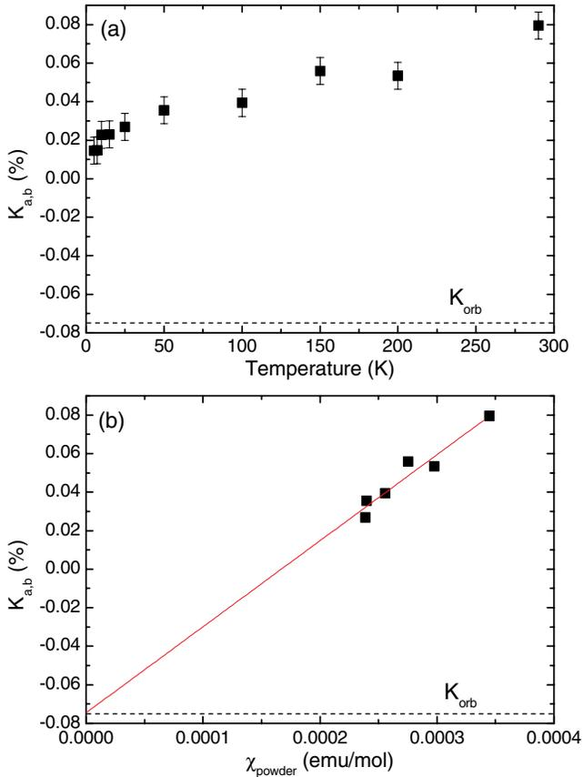
FIG. 3 (color online). (a) Magnetic shift  $K_{ab}$  versus temperature in the aligned sample. The dashed line indicates  $K_{\text{orb}}$ . (b)  $K_{ab}$  versus  $\chi_{\text{powder}}$ , the magnetic susceptibility of the powder sample. The solid line is a fit as described in the text.
