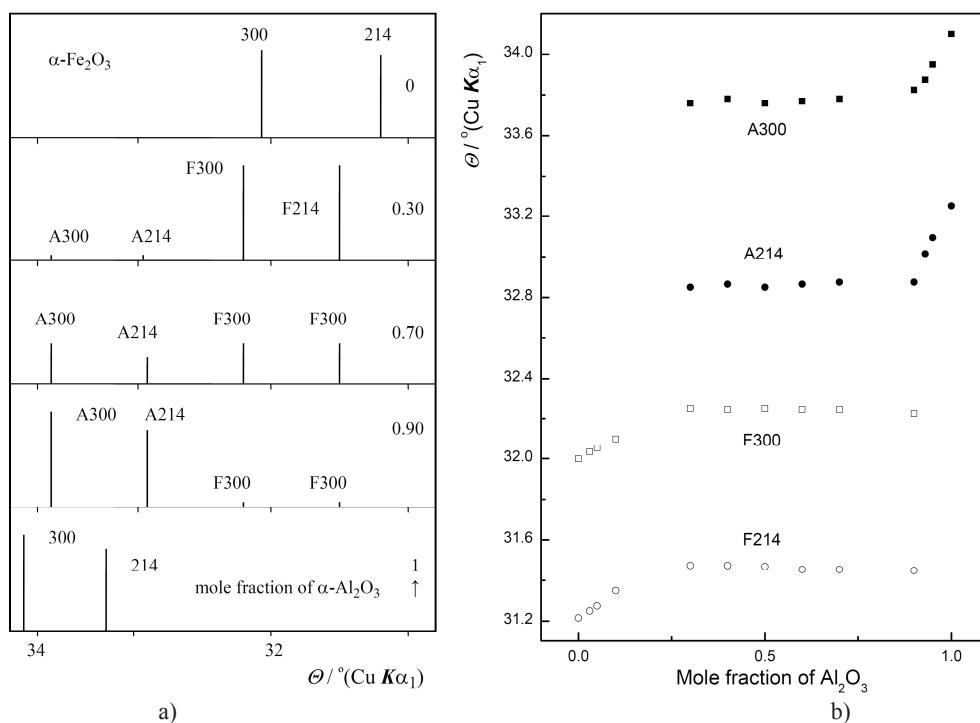
**Figure 1.** a) Schematic representation of Bragg angles  $\Theta$  (Cu  $\mathbf{K}\alpha$ ) and relative intensities of diffraction lines 214 and 300 of phases A and F for samples S0 ( $x = 0$ ), S4 ( $x = 0.30$ ), S8 ( $x = 0.70$ ), S9 ( $x = 0.90$ ) and S12 ( $x = 1$ ). b) The variation of Bragg angles (Cu  $\mathbf{K}\alpha$ ) of diffraction lines 214 and 300 of phases A and F with  $x$ .<sup>14</sup>
