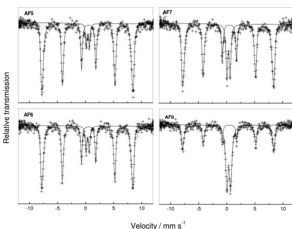
Figure 2. <sup>57</sup>Fe Mössbauer spectra of samples AF5 to AF8 at 20 °C.
