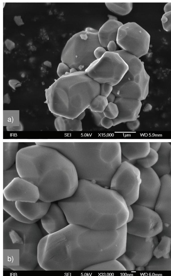
**Figure 7.** FE-SEM image of (a) sample AF10, and (b) sample AF11.
