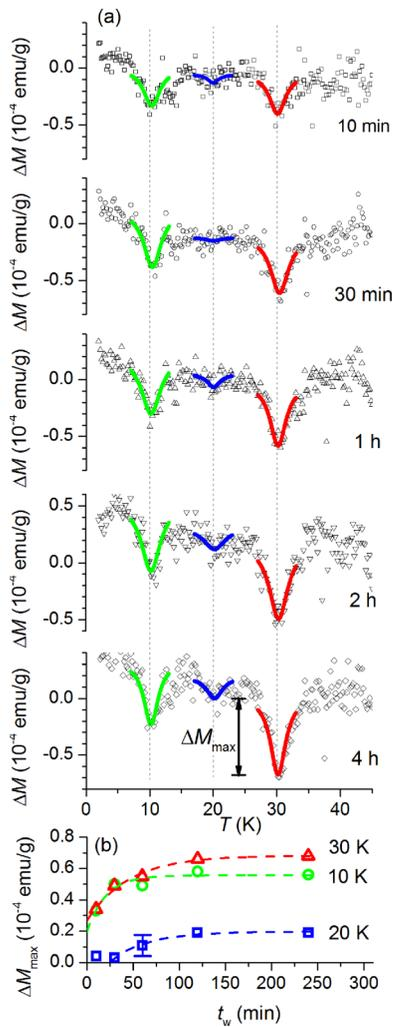
FIG. 2. Memory effect  $\Delta M$  as a function of waiting time  $t_w$  in  $\text{K}_3\text{Cr}_2\text{Fe}_3\text{F}_{15}$  at 10 K, 20 K, and 30 K. (a) The reading field was  $H_r = 4$  Oe. The amplitude of the memory effect  $\Delta M_{\max}$  is plotted versus the waiting time  $t_w$  (b).
