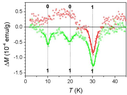
FIG. 3. Three-bit information “111” (lower/green curve) written into  $\text{K}_3\text{Cr}_2\text{Fe}_3\text{F}_{15}$  and another 3-bit information “001” (upper/red curve shifted upward by  $5 \times 10^{-5}$  emu to prevent the two curves from overlapping) after deleting the first two bits. The reading magnetic field was  $H_r = 8$  Oe.
