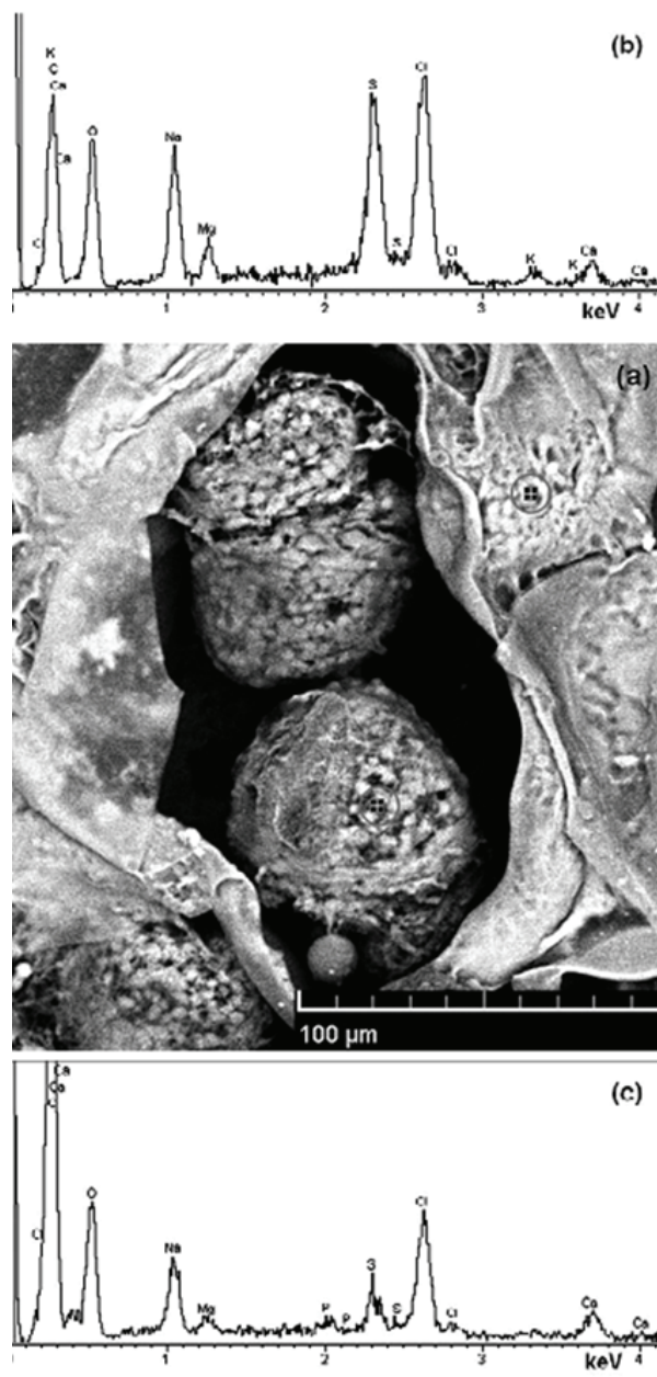
Figure 8. a) ESEM photograph of two embryos (sample C5) in the cocoon. b) EDS pointed to an egg. Contrary to former development stage (sample C4), a clear Ca peak, beside other elements, was observed on the surface of the embryo (sample C5), confirming that the first shell around the embryo was formed. c) EDS pointed to the egg envelope showed organic structure of the tissue.
