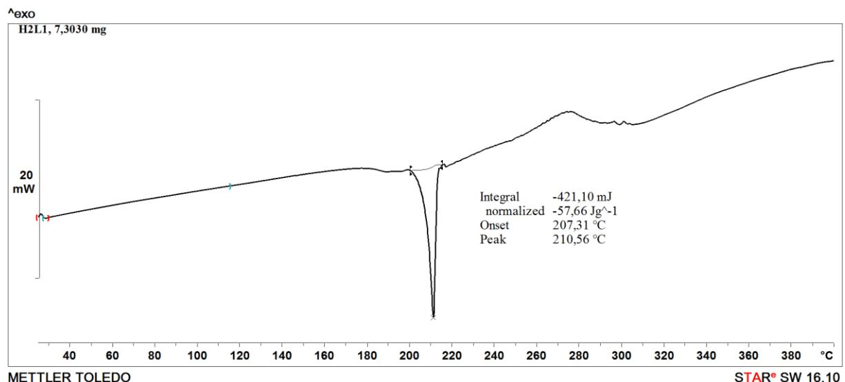
Slika D1. DSC termogram liganda H<sub>2</sub>L<sup>1</sup>
