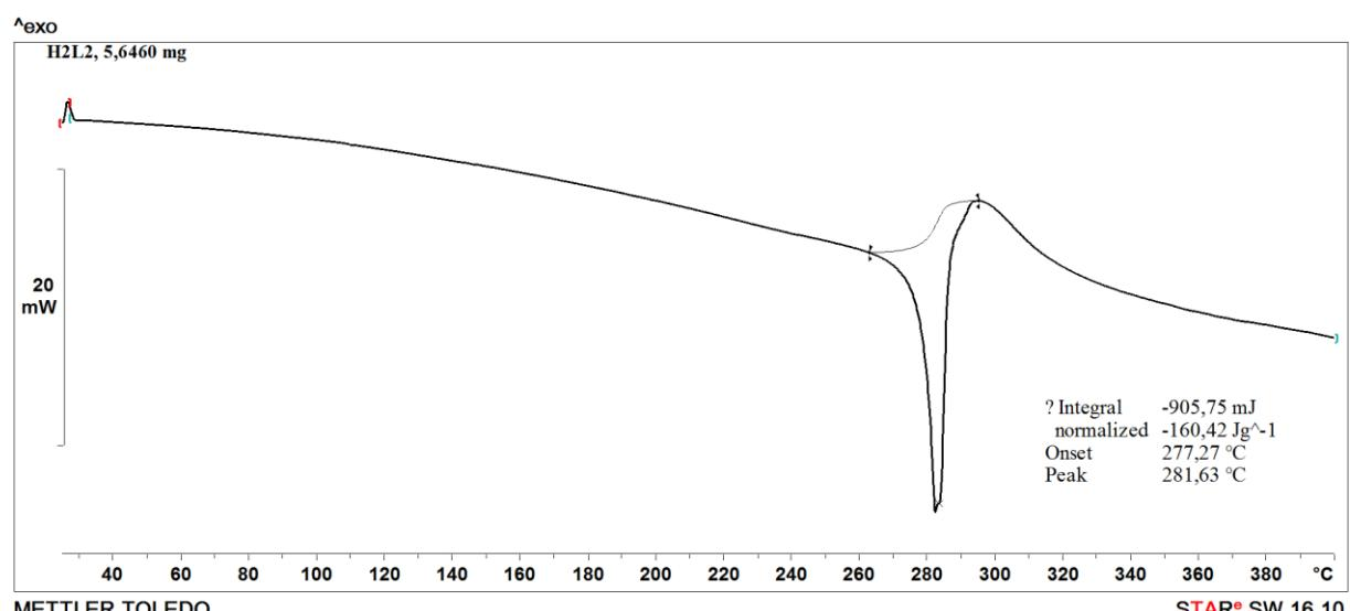
Slika D2. DSC termogram liganda H<sub>2</sub>L<sup>2</sup>
