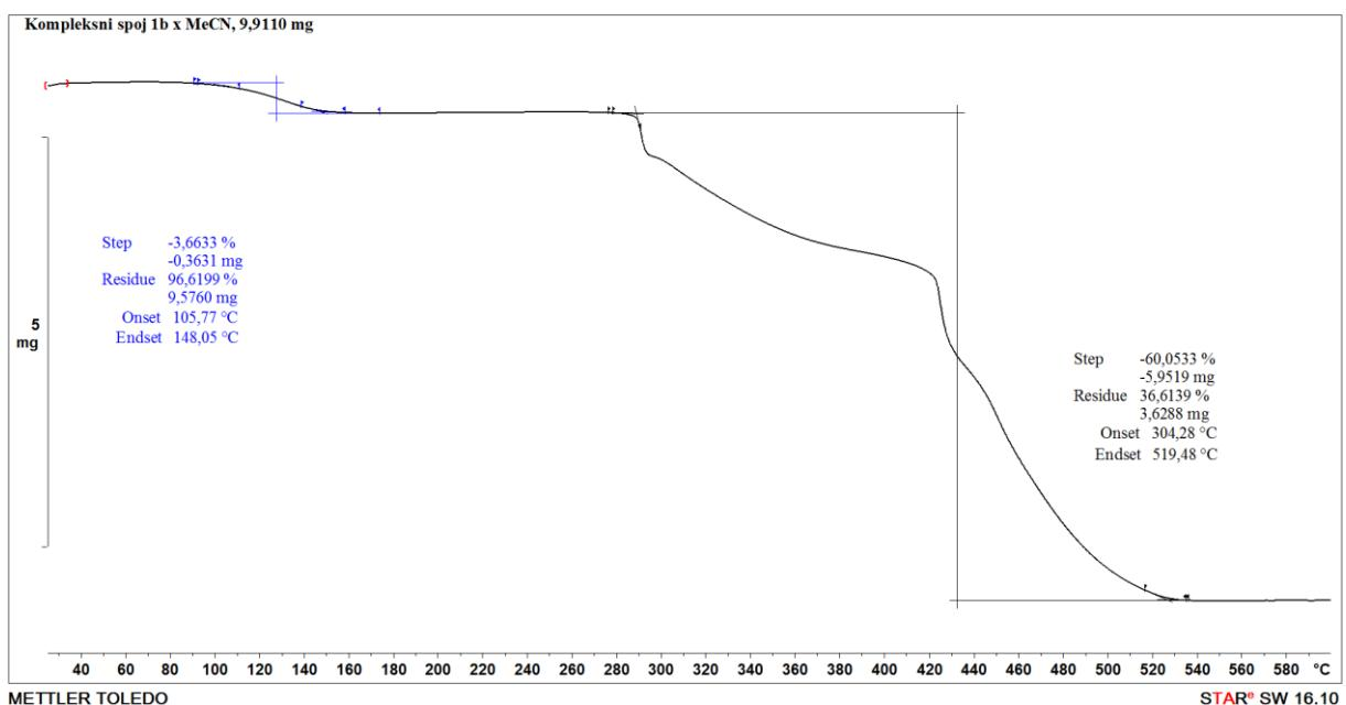
Slika D13. Termogram kompleksnog spoja **1b×MeCN**
