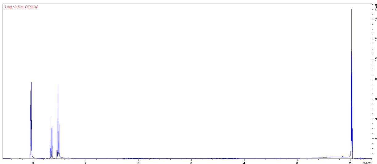
Slika D32. Spektar <sup>1</sup>H NMR standarda benzojeve kiseline ( $\gamma = 5,0 \text{ mg mL}^{-1}$ ) snimljen u acetonitrilu-*d*3 pri 25 °C.
