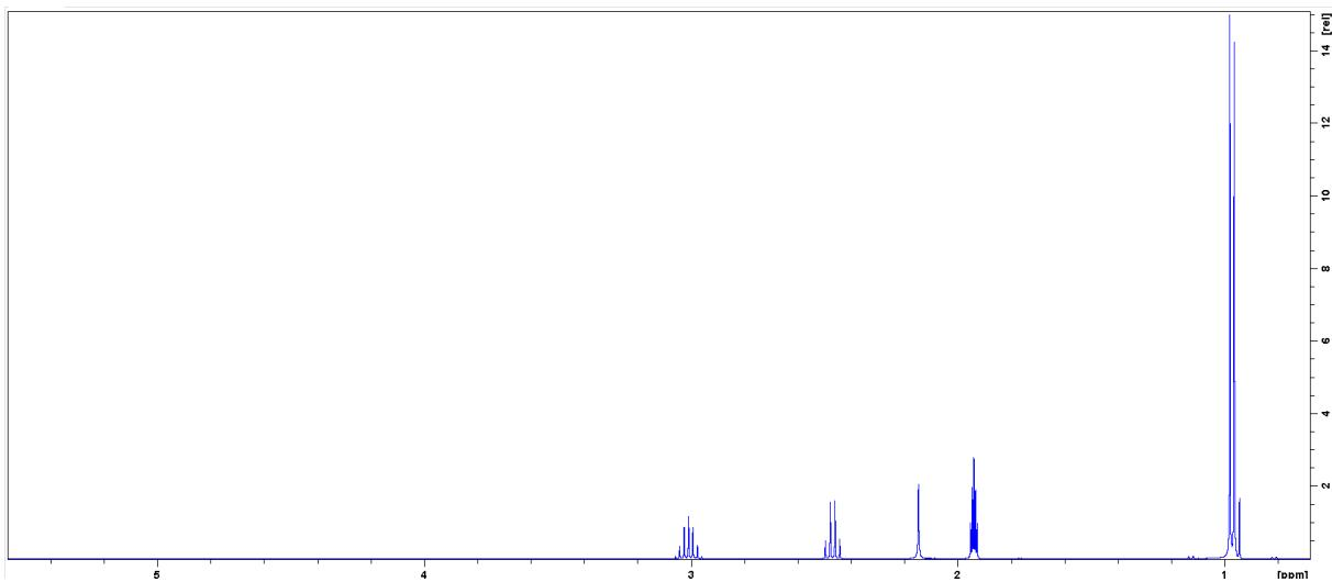
Slika D9. Spektar <sup>1</sup>H NMR DIPEA-e ( $\gamma = 5,0 \text{ mg mL}^{-1}$ ) snimljen u acetonitrilu-*d*3 pri 25 °C.
