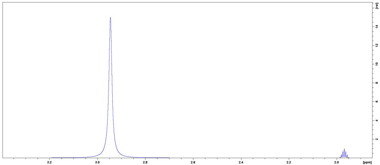
Slika D10. Spektar <sup>1</sup>H NMR hidrazin monohidrata ( $\gamma = 5,0 \text{ mg mL}^{-1}$ ) snimljen u acetonitrilu-*d*3 pri 25 °C.
