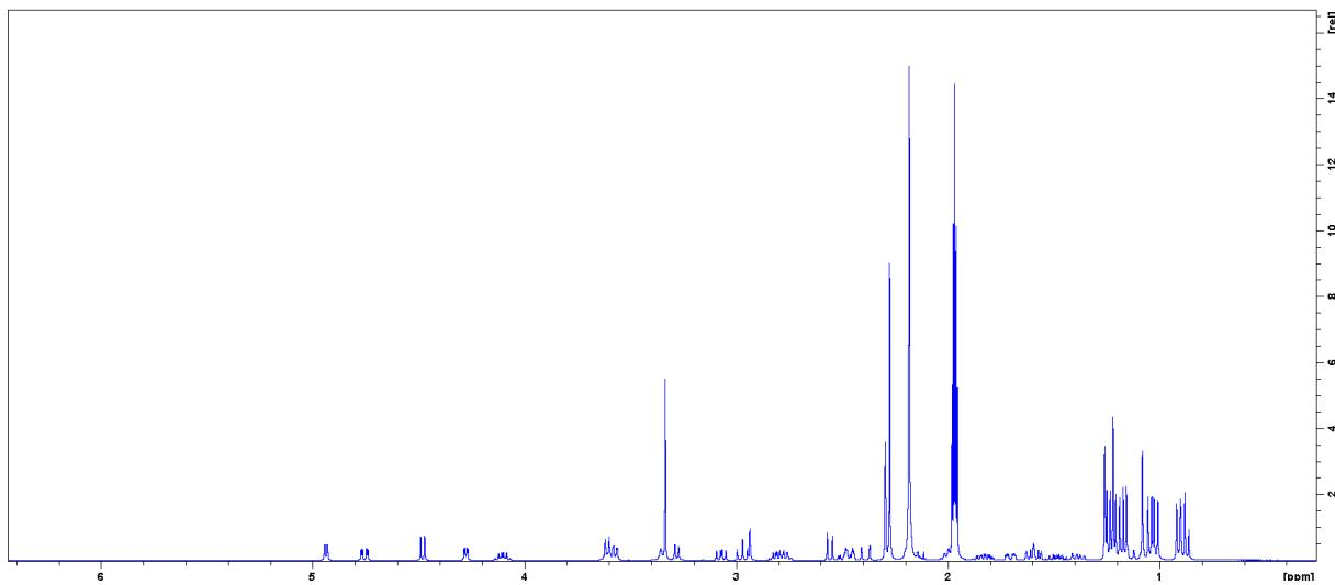
Slika D12. Spektar <sup>1</sup>H NMR azitromicina ( $\gamma = 5,0 \text{ mg mL}^{-1}$ ) snimljen u acetonitrilu-*d*3 pri 25 °C.
