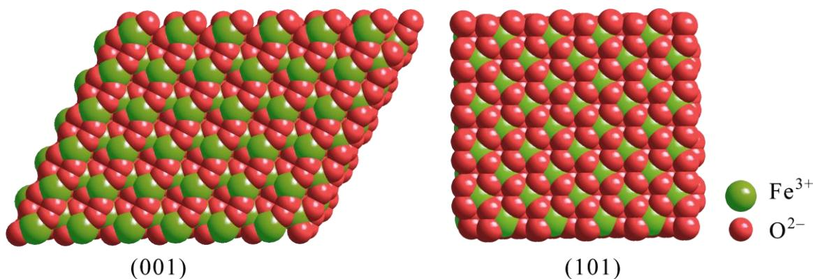
Slika 5.13. Površine hematita,  $\alpha\text{-Fe}_2\text{O}_3$  (001) i (101) nacrtane u programu *Crystal Impact Diamond*.
