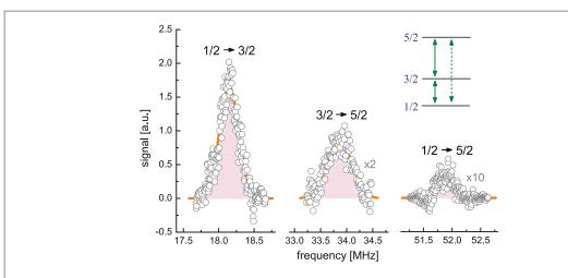
**Figure 1.** NQR signal of  $^{67}$ Zn (spin 5/2) in YBCO-7, at 80 K. All three possible transitions for spin-5/2 NQR were detected, including the 'forbidden' transition  $1/2 \rightarrow 5/2$ , showing that the local EFG at the zinc site is not axially symmetric. For clarity, the  $3/2 \rightarrow 5/2$  and  $1/2 \rightarrow 5/2$  intensities have been magnified by a factor of 2 and 10, respectively.
