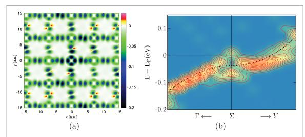
**Figure 5.** (a) Difference of simulated STM images, integrated in a 20 meV window at  $E_f$ , for a slab with  $3 \times 3$  supercell of La<sub>2</sub>CuO<sub>4</sub> unit cells with and without the central Cu replaced by Zn. Note the different densities in the *x*- and *y*-directions. Color scale units:  $10^{-3}a_0^{-3}$ . (b) Spectral function (arbitrary units) near the van Hove singularity for a  $5 \times 5$  supercell, corresponding to 4% Zn doping in the plane.
