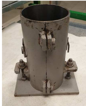
Figure 3.5 Cylindric mould (100 × 200) mm dimensions
