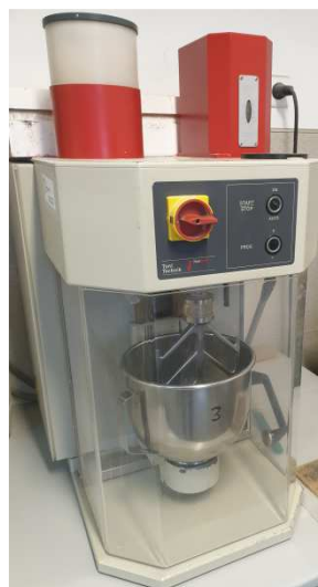
Figure 3.1 Standard mortar mixer
