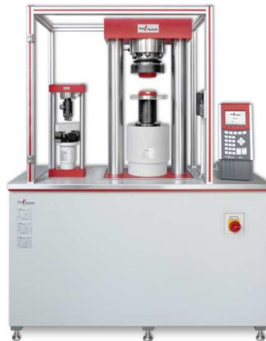
Figure 3.10 The standard strength testing machine
