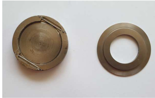
Figure 3.12. Metal holder for in-situ XRD measurements
