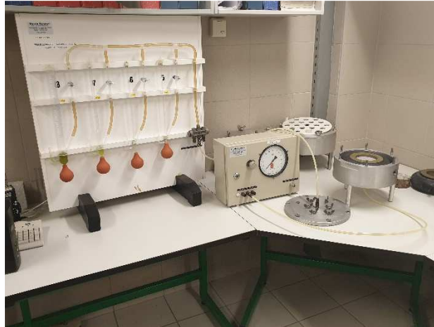
Figure 3.16. The apparatus for determination of permeability to gasses
