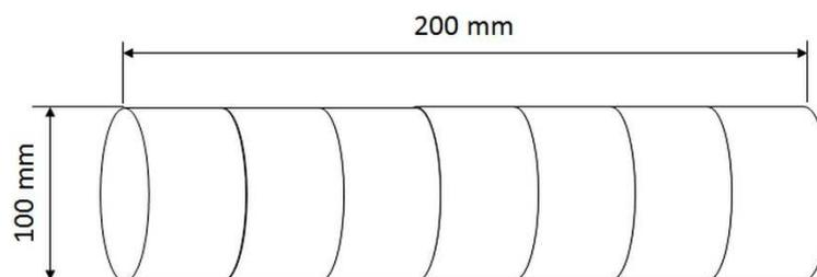
Figure 3.6 Preparation of sub-samples from the cylindrical sample
