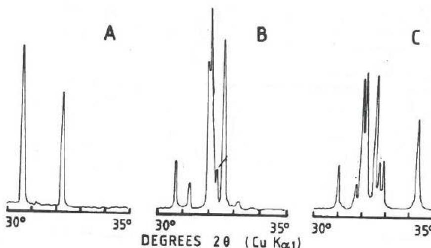
Figure 2.5. XRPD powder patterns of belite modifications from Taylor<sup>5</sup> after Regourd *et al.*<sup>36</sup>
