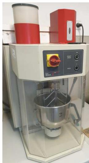
Figure 3.1 Standard mortar mixer
