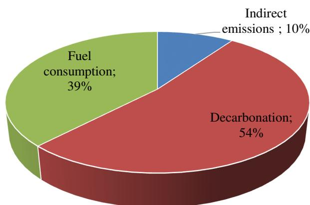
Figure 2.17. Contribution of different sources to CO<sub>2</sub> emissions from Portland cement production<sup>149</sup>
