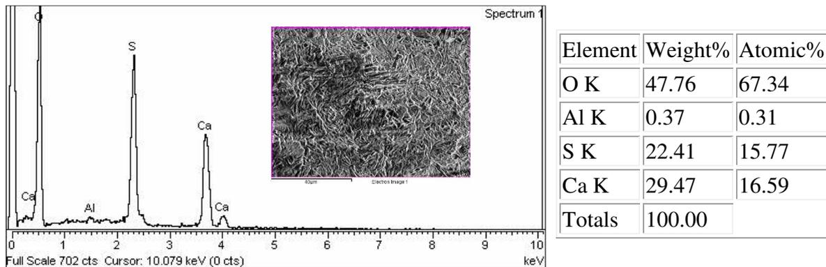
Figure 4.15. EDS spectra of ettringite from the CSA cement paste after leaching
