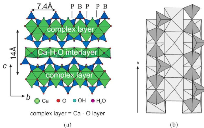
Figure 2.8. Structure of 1.4-nm tobermorite (a) The structure as seen along [100], with two Ca–O layers separated 1.4 nm apart<sup>82</sup> (b) Connection of silicate chains (dark grey) to the layer of calcium polyhedra (light grey), as seen down [100]<sup>83</sup>
