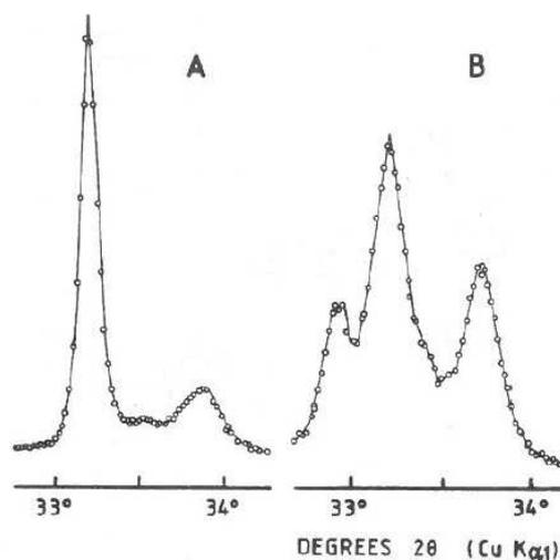
Figure 2.6. XRD powder patterns of aluminate from Taylor<sup>5</sup> after Regourd *et al.*<sup>36</sup>
