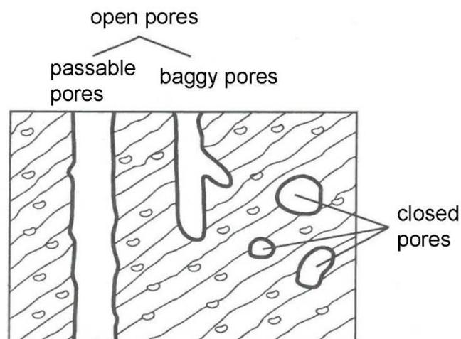
Figure 2.11 Schematic diagrams of pore types in hardened Portland cement paste after Đureković<sup>74</sup>
