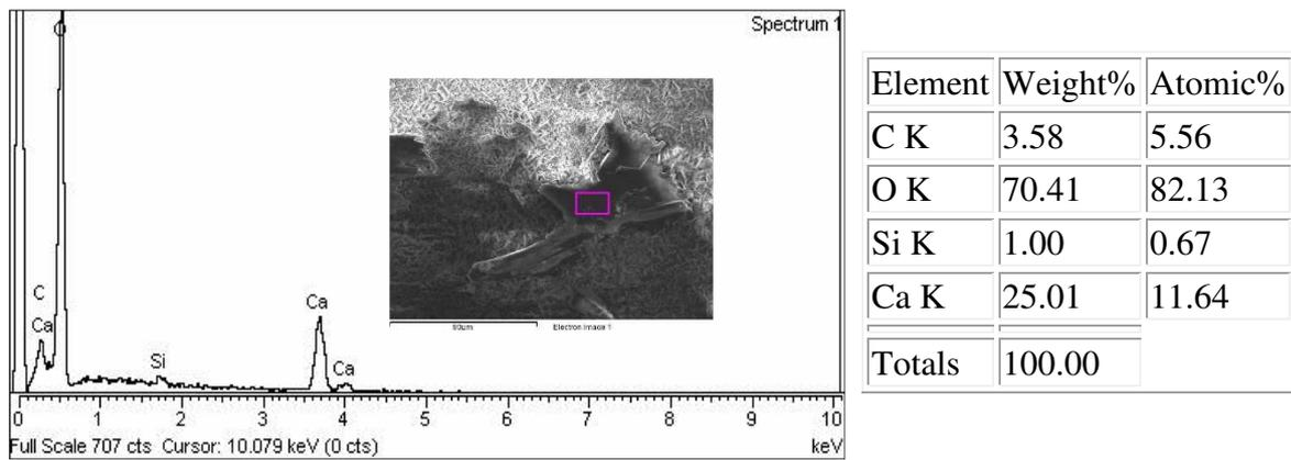
Figure 4.13. EDS spectra of portlandite from the CEM I paste after leaching
