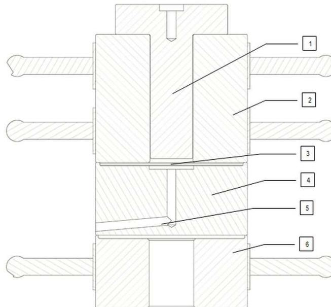
Figure 3.7 Schematic diagram of pore solution expression apparatus
