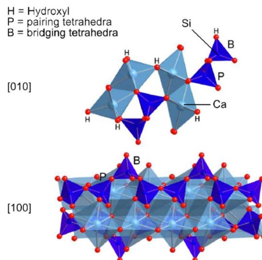
Figure 2.9. Structure of jennite as seen along [010] (top) and [100] (bottom). “H” indicates hydroxyl groups. Reproduced from Richardson who used data from Bonaccorsi<sup>81,84</sup>
