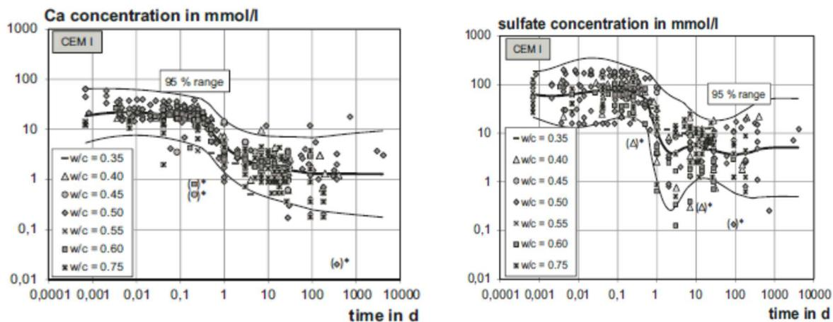
Figure 2.15. Average pore solution concentrations of calcium and sulfate of pure Portland cement pastes after Vollpracht <sup>139</sup>
