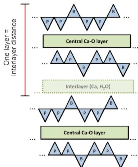
Figure 2.7. Schematic drawing of a dreierketten structure showing the central Ca–O layer and chains of tetrahedral silicates with paired tetrahedra (P) and bridging tetrahedra (B)<sup>79</sup>
