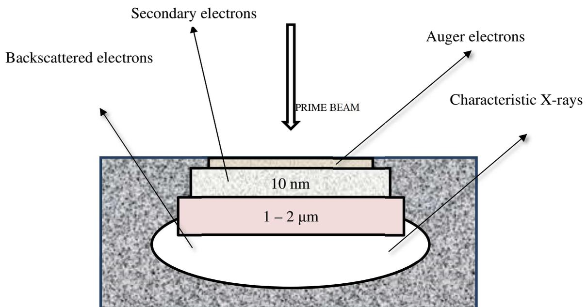
Figure 2.12. Schematic diagram of SEM signals generation
