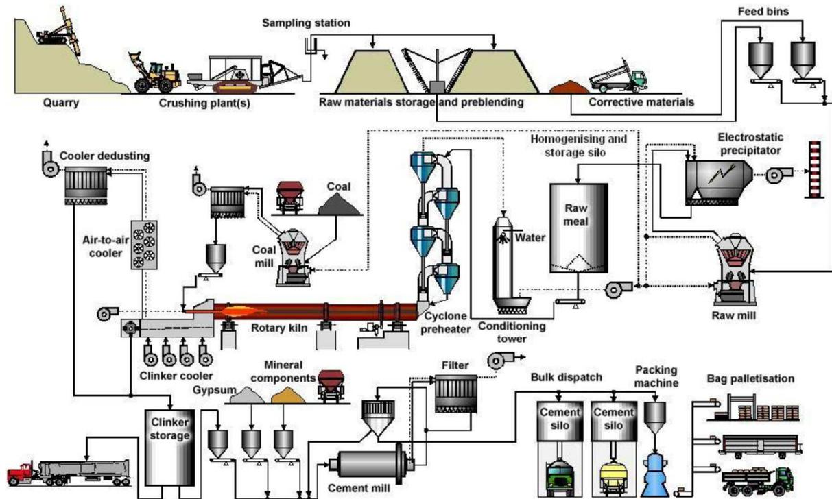
Figure 2.16. General overview of the cement manufacturing process (dry process) after BAT reference document for the production of cement, lime and magnesium oxide<sup>148</sup>
