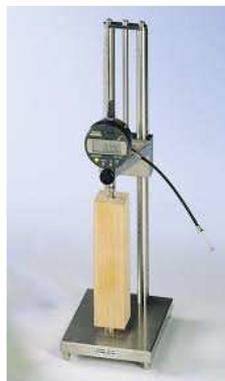
Figure 3.13. Instrument for dimensional stability determination
