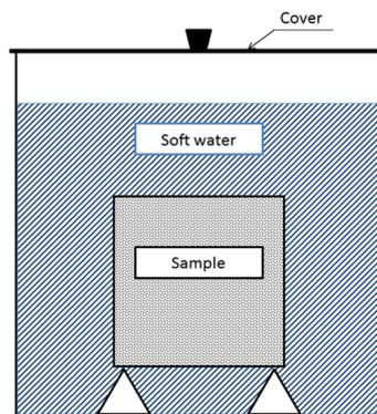
Figure 3.4 Schematic description of tank leaching test
