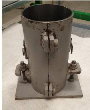
Figure 3.5 Cylindric mould (100 × 200) mm dimensions
