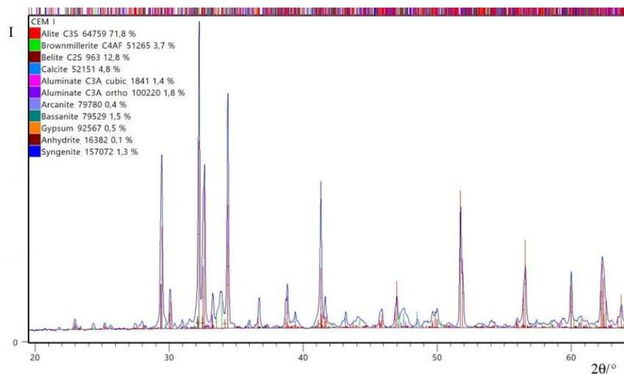
Figure 4.3. QXRPD pattern of CEM I in the  $2\theta$  range 20 – 65°<sup>216-226</sup>
