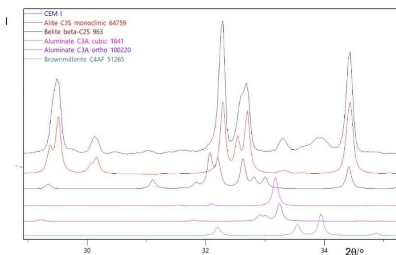
Figure 4.1. XRPD of CEM I in the  $2\theta$  range  $29 - 35^\circ$  with the identified crystalline phases<sup>216-220</sup>
