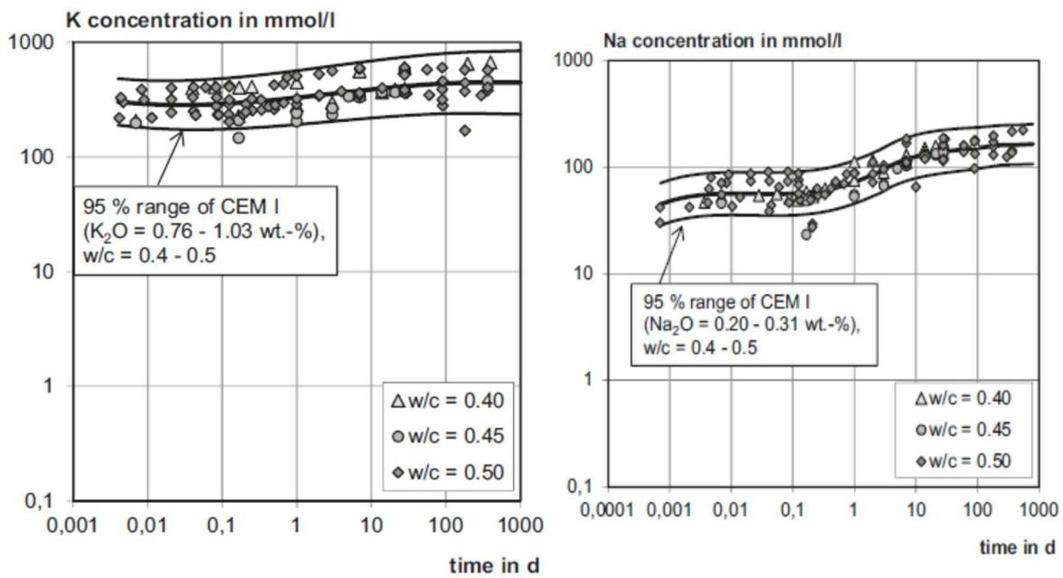
Figure 2.13. Average pore solution concentrations of potassium and sodium in pure Portland cement pastes with K<sub>2</sub>O content between 0.76 % - 1.03 % and Na<sub>2</sub>O content between 0.20 % - 0.31 %, after Vollpracht *et al.*<sup>139</sup>
