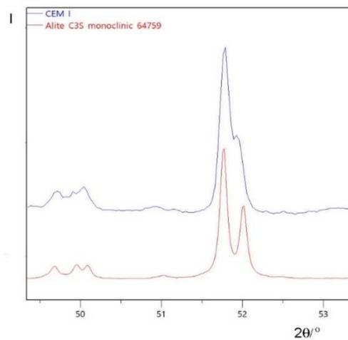
Figure 4.2. Characteristic XRPD pattern of the observed monoclinic  $M_1$  alite polymorph in CEM I (top) and the calculated pattern of the  $M_3$  polymorph (bottom)<sup>216</sup>
