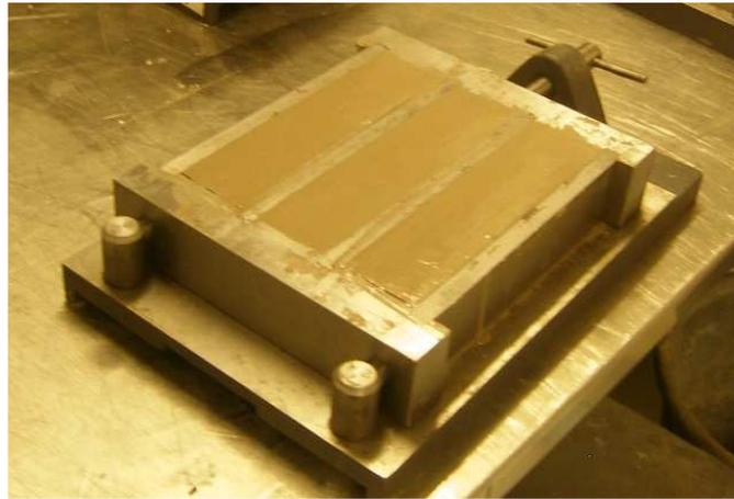
Figure 3.2 Filled standard prismatic moulds
