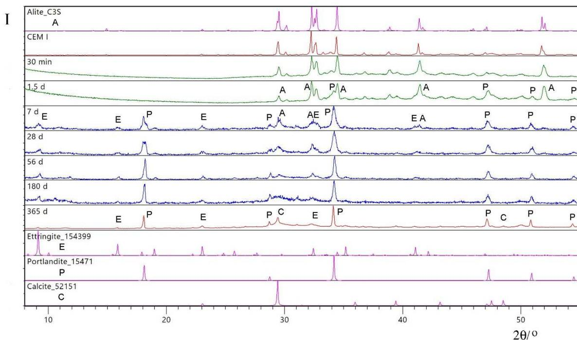
Figure 4.6. XRPD of CEM I cement paste in the  $2\theta$  range  $8 - 55^\circ$ . Observed powder patterns for CEM III and the CEM III paste after 365 days of hydration and leaching are shown red
