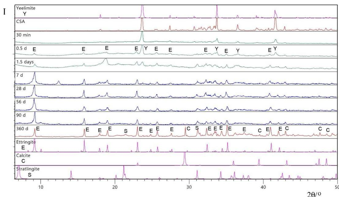
Figure 4.8. XRPD of CSA cement paste in the  $2\theta$  range  $8 - 55^\circ$  with the identified crystalline phases.<sup>216,221,235-236</sup> Calculated powder patterns of known crystal structures are shown in pink color. Observed powder patterns for CSA cement and the CSA cement paste after 365 days of hydration and leaching are shown red color. *In-situ* patterns are shown in green color. Patterns of hydrated and leached CSA cement paste are shown in blue color. known crystal structures
