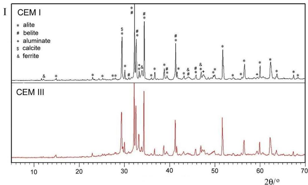
Figure 4.4. XRPD of CEM III in the  $2\theta$  range 9 – 65° with the identified crystalline phases<sup>216-218,220,221</sup>
