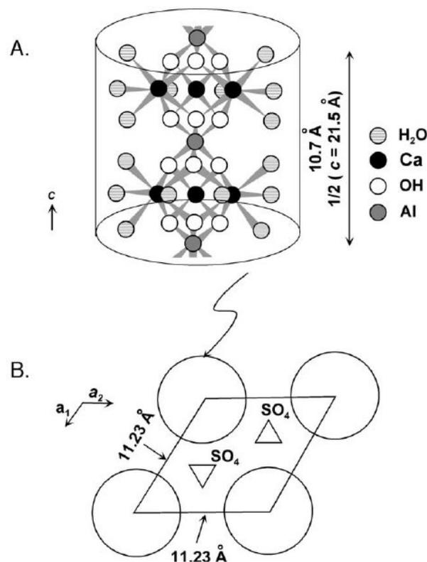
Figure 2.10. Schematic structure of ettringite after Taylor<sup>107</sup>
