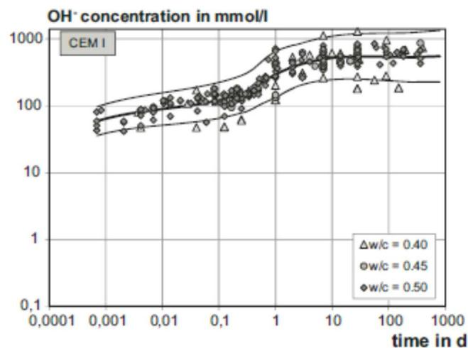
Figure 2.14. Average pore solution concentrations of  $\text{OH}^-$  ions of pure Portland cement pastes after Vollpracht <sup>139</sup>
