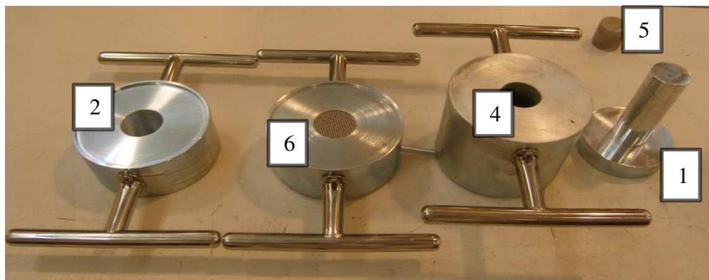
Figure 3.8 Parts of pore solution expression apparatus
