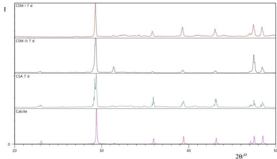
Figure 4.9 *In-situ* XRPD of CEM I, CEM III and CSAC cement pastes in the  $2\theta$  range  $8 - 55^\circ$  <sup>221</sup>
