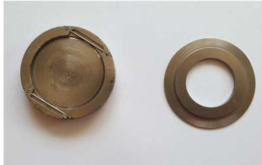
Figure 3.12. Metal holder for in-situ XRD measurements
