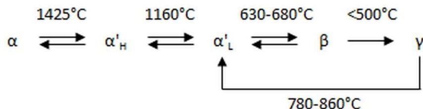
Figure 2.3. Temperature phase transformations of pure  $\text{C}_2\text{S}$  after Taylor<sup>5</sup>
