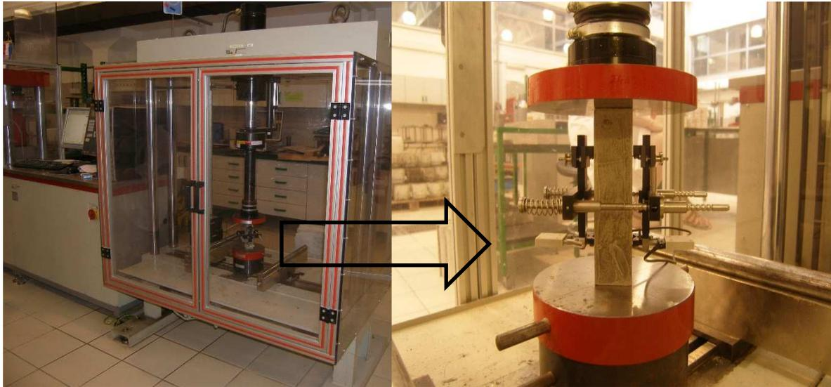
Figure 3.11. Determination of secant modulus of elasticity
