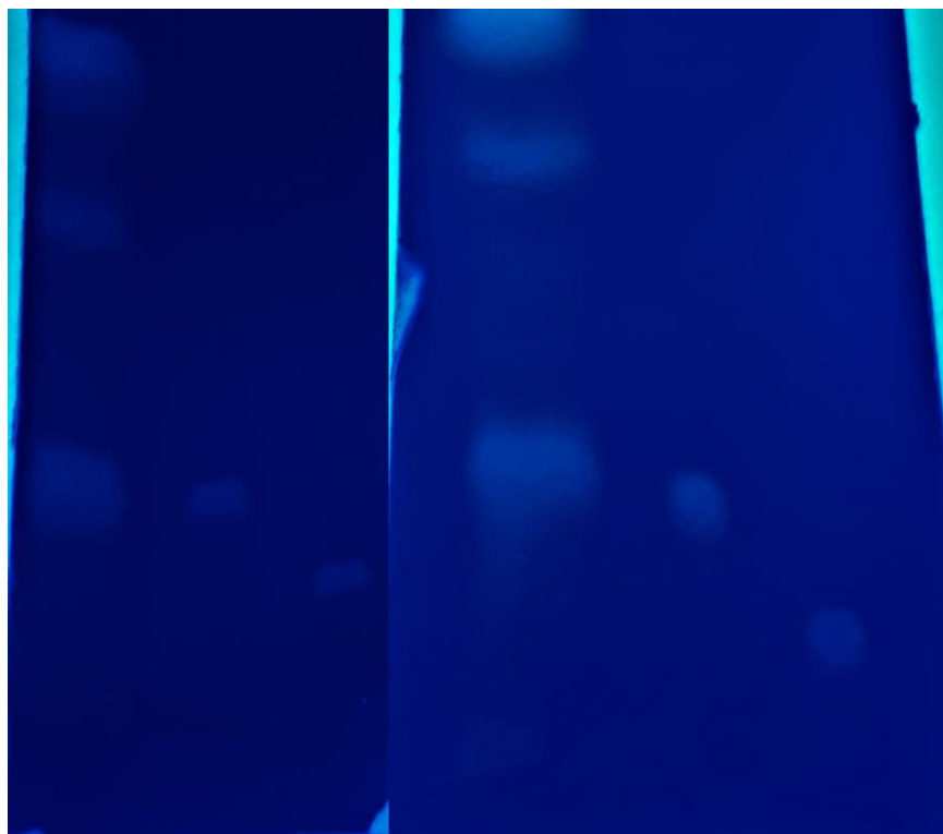
Figure 14 Analytical TLC of (from left to right) non-polar lipid extract, triolein standard and TG-estolide standard, a) Left TLC plate developed with Hexane: Diethyl ether: formic acid = 92.5:7.5:2, b) Right TLC plate developed with Hexane: Diethyl ether = 92.5:7.5
