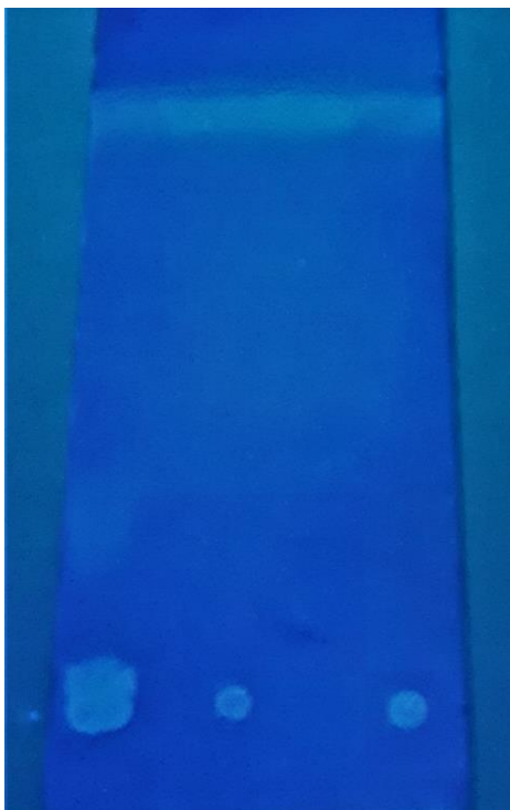
Figure 12 Analytical TLC of (from left to right) non-polar lipid extract, triolein standard and TG-estolide standard, solvent system \rightarrow Hexane: formic acid = 100:2
