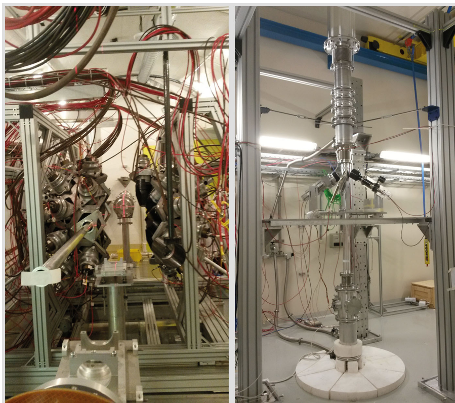
Fig. 4. Picture of the horizontal neutron beam line in EAR1 (left panel) showing the TAC in open position, and the vertical neutron beam line in the newly constructed EAR2 (right panel), showing a neutron capture setup with C_6D_6 detectors above the chamber containing the silicon neutron beam monitors (SiMon2).
