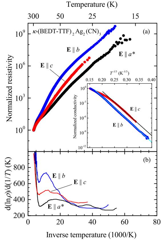
FIG. 7. (a) DC resistivity normalized to room temperature value and (b) logarithmic resistivity derivative of  $\kappa$ -AgCN versus inverse temperature. The inset displays the normalized dc conductivity as a function of  $T^{-1/3}$ ; the behavior evidences the variable-range hopping in two dimensions, whereas above about 140 K, the behavior crosses over into the nearest-neighbor hopping described by a simple activation.
