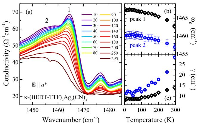
FIG. 2. (a) Temperature evolution of the intramolecular vibration  $\nu_{27}$  in  $\kappa$ -AgCN. The two Fano functions required to fit the spectra indicate two crystallographically distinct sites. No effect on cooling rate (0.1 and 1 K/min) was observed. Temperature dependence of the (b) resonance frequency and (c) damping.
