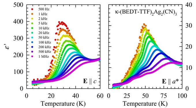
FIG. 3. Real part of the dielectric function  $\epsilon'$  of  $\kappa$ -AgCN as a function of temperature. The frequency dependent measurements performed with the ac electric field applied  $\mathbf{E} \parallel c$  (left panel) and  $\mathbf{E} \parallel a^*$  (right panel) both demonstrate the relaxor-ferroelectric behavior.
