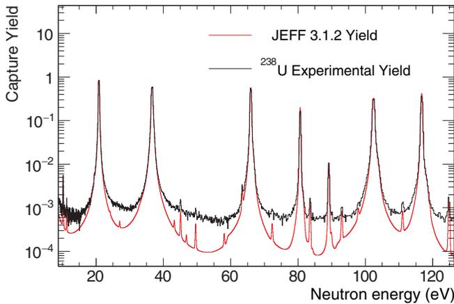
FIG. 6. The  $^{238}\text{U}$  experimental yield after initial background subtraction compared to the calculated yield from SAMMY using resonance parameters from JEFF 3.1.2. A small background still remains within the data, which can be quantified by finding the required normalization to match the data to what is expected as a function of neutron energy.
