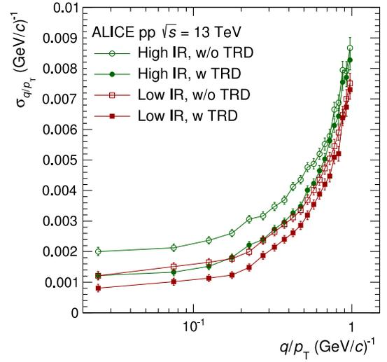
Fig. 27. Improvement of the  $q/p_T$  resolution in data when TRD information is included as compared with the performance of tracking without TRD information for various running scenarios. The labels low and high IR indicate interaction rates of 12 and 230 kHz, respectively.
