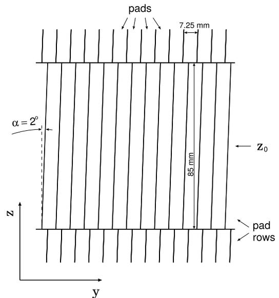
Fig. 4. Pad geometry of a TRD read-out chamber in layer 3 (not stack 2). The pad tilt is  $\pm 2^\circ$  with respect to the  $z$ -axis (along the beam direction), with the sign alternating between layers.
