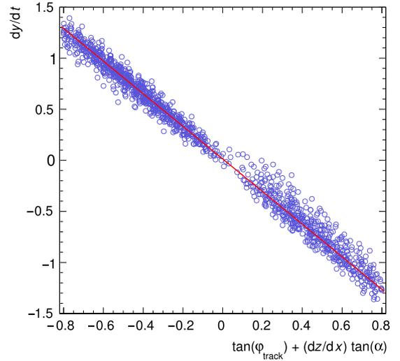
Fig. 34. The derivative of the local tracking  $y$  coordinate with respect to the drift time  $t$  vs. the tangent of the azimuthal track inclination angle from global tracking. The slope and the offset of the fit (red line) give the drift velocity and the Lorentz angle, respectively.
