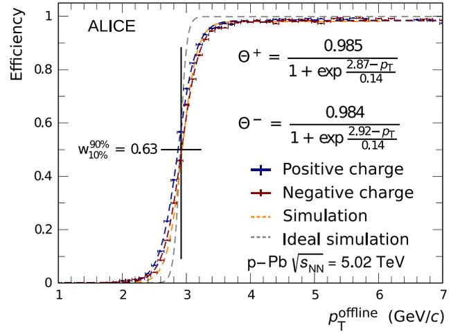
**Fig. 53.** Turn-on curve of the trigger with a  $p_T$  threshold of 3 GeV/c for positively and negatively charged particles in comparison to the same variable computed in simulation with a realistic detector geometry (active channels). Also shown is the corresponding distribution for an ideal detector geometry (ideal simulation, not considering misalignment). The onset is characterised by a fit with a Fermi function.
