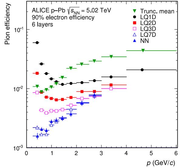
Fig. 43. Pion efficiency (for 90% electron efficiency) as a function of momentum for the truncated mean, LQ1D, LQ2D, LQ3D, LQ7D and NN methods. The results are from p–Pb collisions at  $\sqrt{s_{\text{NN}}} = 5.02$  TeV and for tracks with signals in six layers.
