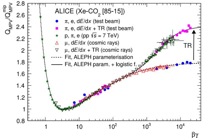
Fig. 37. Most probable charge deposit signal normalised to that of minimum ionising particles as a function of  $\beta\gamma$ . The data are from measurements performed in test beam runs, pp collisions at  $\sqrt{s} = 7$  TeV, and cosmic-ray runs. Uncertainties in momentum and thus  $\beta\gamma$  determination are drawn as horizontal and statistical uncertainties as vertical error bars. The shown fits correspond to Eqs. (1) and (2) described in the text.
