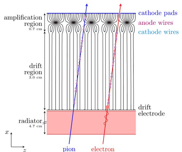
Fig. 2. Schematic cross-section of a TRD chamber in the  $x$ - $z$  plane (perpendicular to the wires) with tracks of a pion and an electron to illustrate the ionisation energy deposition and the TR contribution. The large energy deposition due to the TR photon absorption is indicated by the large red circle in the drift region. The drift lines (solid lines) are calculated with Garfield [43] and correspond to the nominal voltage settings for chamber operation. The radiator is not drawn to scale.
