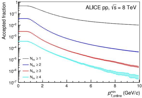
**Fig. 54.** Rejection by the level-1 trigger for requiring 1–4 tracks in any stack ( $N_{\text{trk}}$ ) above varying  $p_T$  thresholds for pp collisions at  $\sqrt{s} = 8$  TeV [70]. The error bars indicate the statistical uncertainties. The distributions were obtained by counting the number of tracks in a stack above a given threshold and normalised by the number of sampled events.
