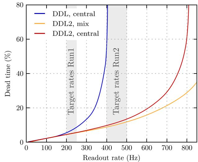
**Fig. 16.** Simulation of the dead time as function of the read-out rate in Pb–Pb collisions for the effective DDL bandwidth in Run 1 (DDL) and Run 2 (DDL2). The simulation assumes a 5% L1/L0 accept ratio and no L2 rejects. The scenarios central and mix correspond to an event size of 470 kB and 310 kB per supermodule, respectively, mimicking thus different event multiplicities.
