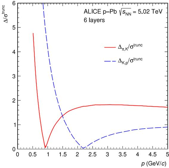
Fig. 40. Measured separation power ( $\frac{\Delta}{\sigma^{\text{trunc}}} = \frac{S_{\pi/K}^{\text{trunc}} - S_{\pi/K}^{\text{trunc}}}{\sigma^{\text{trunc}}}$ ) for  $\pi/K$  and  $K/p$  separation as a function of momentum.
