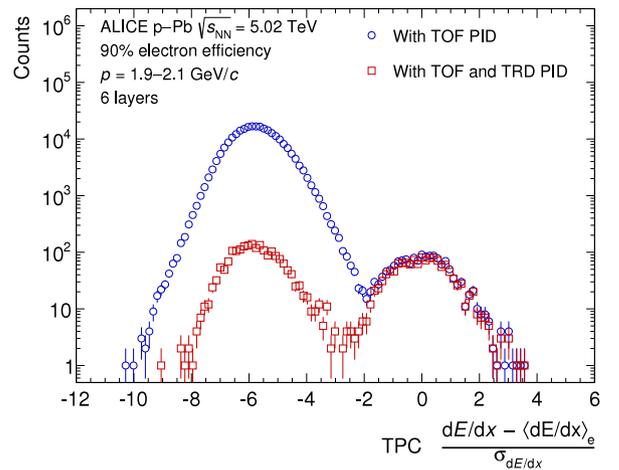
Fig. 44. Difference in units of standard deviations between the measured TPC energy loss of a given track and the expected energy loss of an electron with TOF ( $\pm 3\sigma_e^{\text{TOF}}$ ) and TRD (90% electron efficiency) electron identification. The distributions are shown for tracks with a momentum of 1.9–2.1 GeV/c within the TRD acceptance (6 layers in the TRD) in p–Pb collisions at  $\sqrt{s_{\text{NN}}} = 5.02$  TeV.
