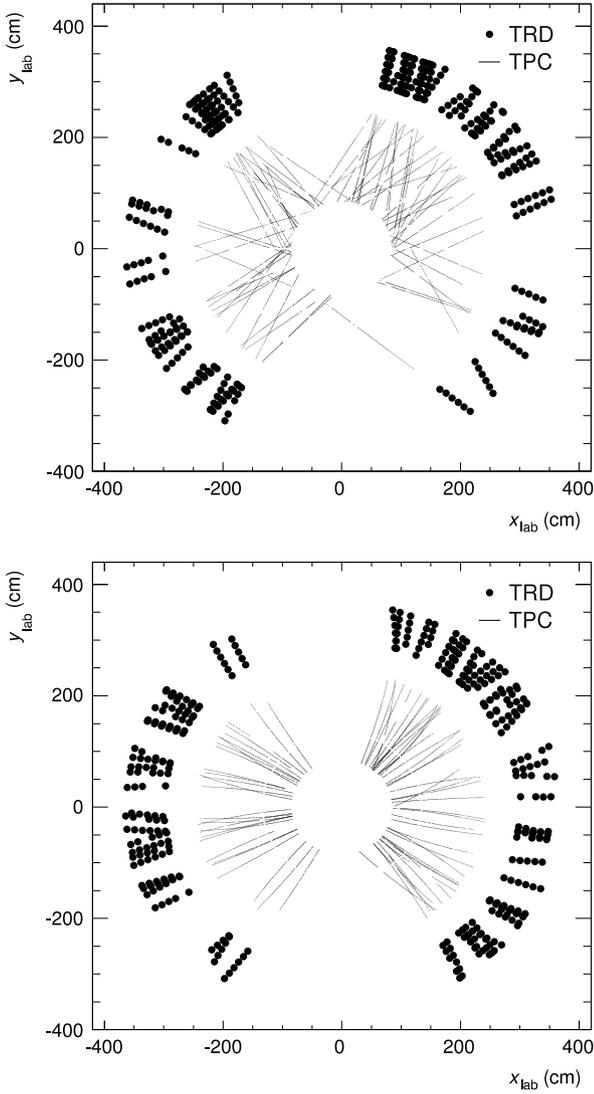
**Fig. 28.** Top: Cosmic-ray tracks with at least 100 TPC clusters and 5 TRD layers, recorded without magnetic field, used for the relative  $r\phi$  alignment of the TRD chambers within stacks (internal alignment). Bottom: Charged-particle tracks with at least 100 TPC clusters and 4 TRD layers from pp collisions at  $\sqrt{s} = 8$  TeV, used for the alignment of the TRD with respect to the TPC (external alignment). Both figures show data from 2012 (setup with 13 supermodules).
