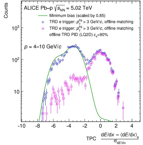
Fig. 58. Electron selection for triggered data with and without the TRD offline PID (see Section 11) in Pb–p collisions at  $\sqrt{s_{NN}} = 5.02$  TeV. Electrons from photon conversions in the detector material were rejected by matching the online track with a track in the TPC. The corresponding distribution for minimum-bias data, scaled to the maximum of the distribution of the triggered data sample, is shown to visualise the TRD trigger capability to enhance electrons.
