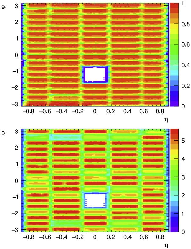
Fig. 35. Two quality-assurance plots (data from pp collisions recorded in 2015 with all supermodules installed, tracks with at least 70 TPC clusters and  $p_T > 0.5$  GeV/c). Top: Efficiency of matching tracklets to TPC tracks. Bottom: Mean number of layers per track in each stack (cf. the discussion of inactive chambers in Section 7.2).
