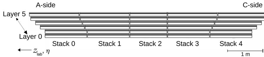
Fig. 3. Cross-section (longitudinal view) of a supermodule.
