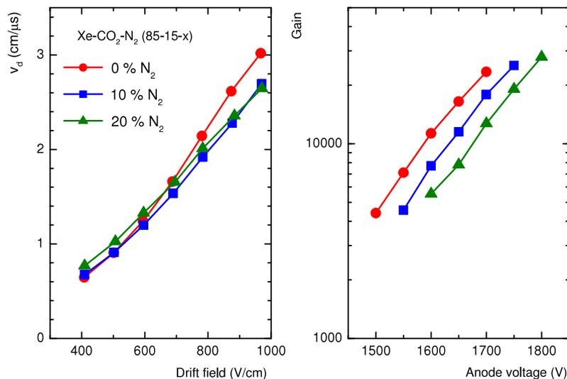
Fig. 11. Left: Drift velocity as a function of the drift field for the nominal gas mixture Xe-CO<sub>2</sub> and different admixtures of N<sub>2</sub>. Right: Gain as a function of the anode voltage for the same gas mixtures.
