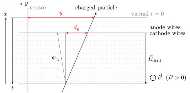
Fig. 46. Sketch of the tracklet reconstruction. The tracklet reconstruction in the MCMs is performed in a local coordinate system. The tracklet comprises the information on  $y$ ,  $d_y$ ,  $z$  and PID. The magnetic and electric field and the effect of the Lorentz angle ( $\Psi_L$ ) are indicated as well.
