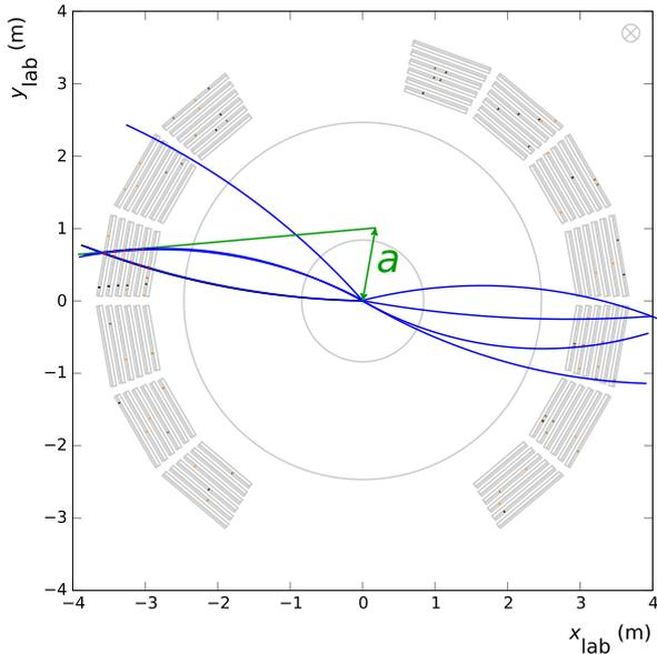
**Fig. 48.** Event display showing the tracks available for the level-1 trigger from the online reconstruction (green) in comparison with helix fits to the contributing tracklets (blue). The offset  $a$  from the primary vertex used as measure for  $1/p_T$  is shown as well. The colour coding of the tracklets (small boxes) is according to stacks. (For interpretation of the references to colour in this figure legend, the reader is referred to the web version of this article.)
