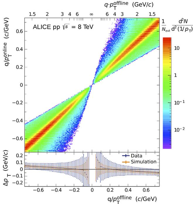
**Fig. 52.** Top: Correlation between  $1/p_T$  obtained from the online tracking and from a matched offline track for pp collisions at  $\sqrt{s} = 8$  TeV. Bottom: Difference (points) of the online and offline track  $p_T$  for data and simulation. The error bars indicate the corresponding width of the difference in  $p_T$ .
