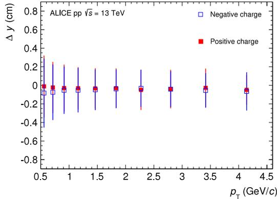
Fig. 23. Residuals in  $\Delta y$  of tracklets with respect to global tracks as a function of  $p_T$  in pp collisions at  $\sqrt{s} = 13$  TeV. For every bin the mean (marker) and r.m.s. width (error bar) of the distribution are shown.
