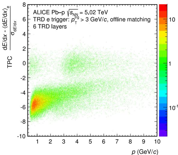
Fig. 57.  $n_{\sigma_{TPC}}$  as a function of momentum for Pb–p collisions at  $\sqrt{s_{NN}} = 5.02$  TeV recorded with the electron trigger ( $p_T$  threshold at 3 GeV/c). Electrons from photon conversions in the detector material were rejected by matching the online track with a track in the TPC.
