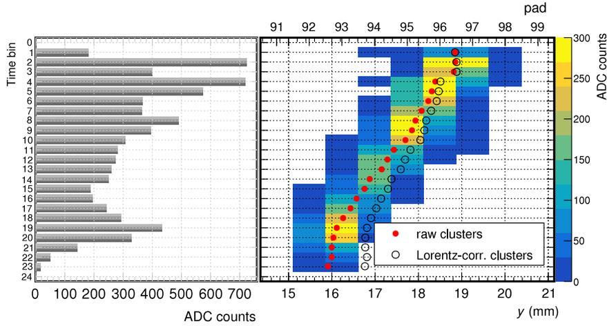
Fig. 22. Signal produced by a positively charged particle ( $p_T = 0.5$  GeV/c). Left: Total charge per time bin used for particle identification. Right: Ionisation signal vs. pad number and time bin. The cluster positions are shown as reconstructed from the charge distribution (raw clusters) and after correction for the  $E \times B$  effect (Lorentz-corr. clusters).
