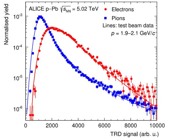
Fig. 36. Total integrated charge, normalised to the tracklet length, measured in a single read-out chamber for electrons and pions in p–Pb collisions at  $\sqrt{s_{NN}} = 5.02$  TeV, in comparison with results from test beam measurements (solid lines) [47,105]. The electrons and pions from test beam measurements were scaled by one common factor to compensate the difference in gain of the two data sets.
