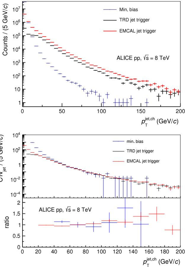
**Fig. 55.** Top:  $p_T$  spectra of leading jets for the minimum-bias and triggered samples of pp collisions at  $\sqrt{s} = 8$  TeV [70]. The leading jets are defined as the jets with the highest  $p_T$  in the event. Bottom: For comparison the  $p_T$  spectra were scaled to the same yield between 60 and 80 GeV/c. The spectra were re-binned to calculate the ratios.
