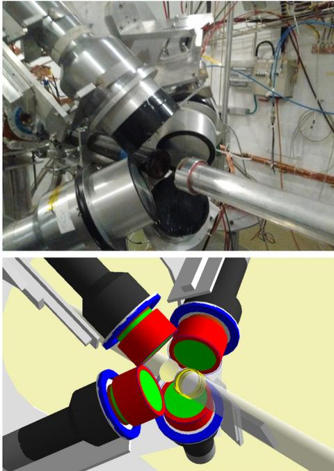
FIG. 2. Top: Array of four C<sub>6</sub>D<sub>6</sub> detectors used to detect the  $\gamma$ -ray cascades emitted following the neutron capture on the  $^{242}\text{Pu}$  sample. Bottom: Geometry implemented in GEANT4 to simulate the response of the detection setup.
