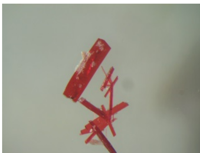
Slika 23: Fotografija jediničnog kristala kompleksa [\text{Co}^{\text{III}}\text{C}_2\text{O}_4(\text{NH}_3)_4]_2[\text{Co}^{\text{II}}(\text{C}_2\text{O}_4)_2(\text{H}_2\text{O})_2]\cdot 4\text{H}_2\text{O} .
