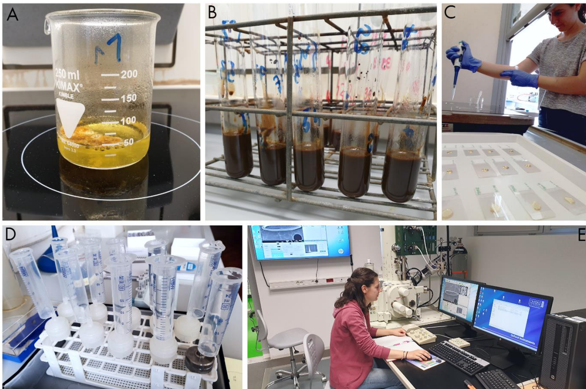
Figure 11. Light and electron microscopy and sample preparation. A – cleaning carapace sample from organic matter in HNO 3 . B – cleaning culture samples in KMnO 4 . C – preparing permanent microscopic slides for LM (photo: A. Žiroš). D – preparing samples on filters for SEM. E – observing samples on SEM (photo: S. Bosak).
