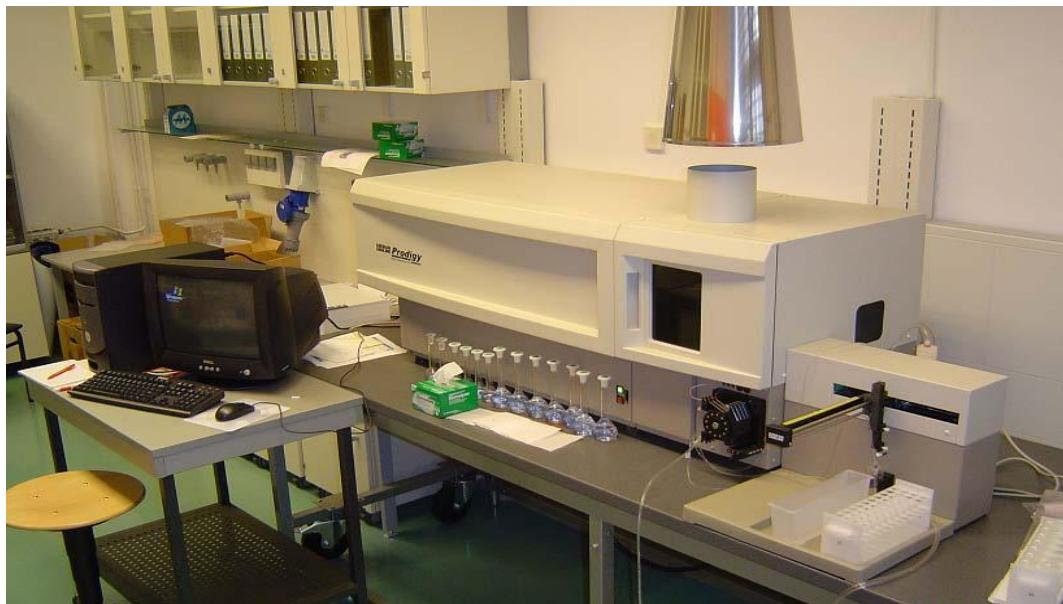
Slika 9. Spektrometar *Prodigy High Dispersive ICP*.
