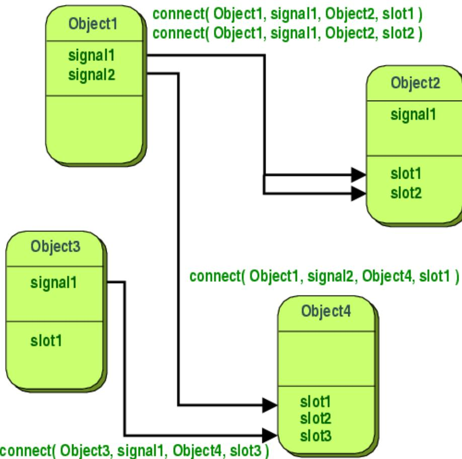
Slika 5. Signals and slots primjer (<https://doc.qt.io/qt-5/signalsandslots.html>)
