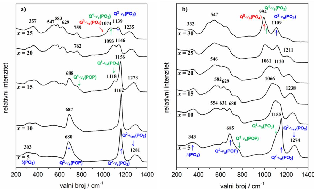
Slika 33. Ramanovi spektri za stakla iz serija C:  $40\text{Na}_2\text{O}-(60-x)\text{P}_2\text{O}_5-x\text{GeO}_2$  (a) i D:  $40\text{Na}_2\text{O}-10\text{B}_2\text{O}_3-(50-x)\text{P}_2\text{O}_5-x\text{GeO}_2$  (b).
