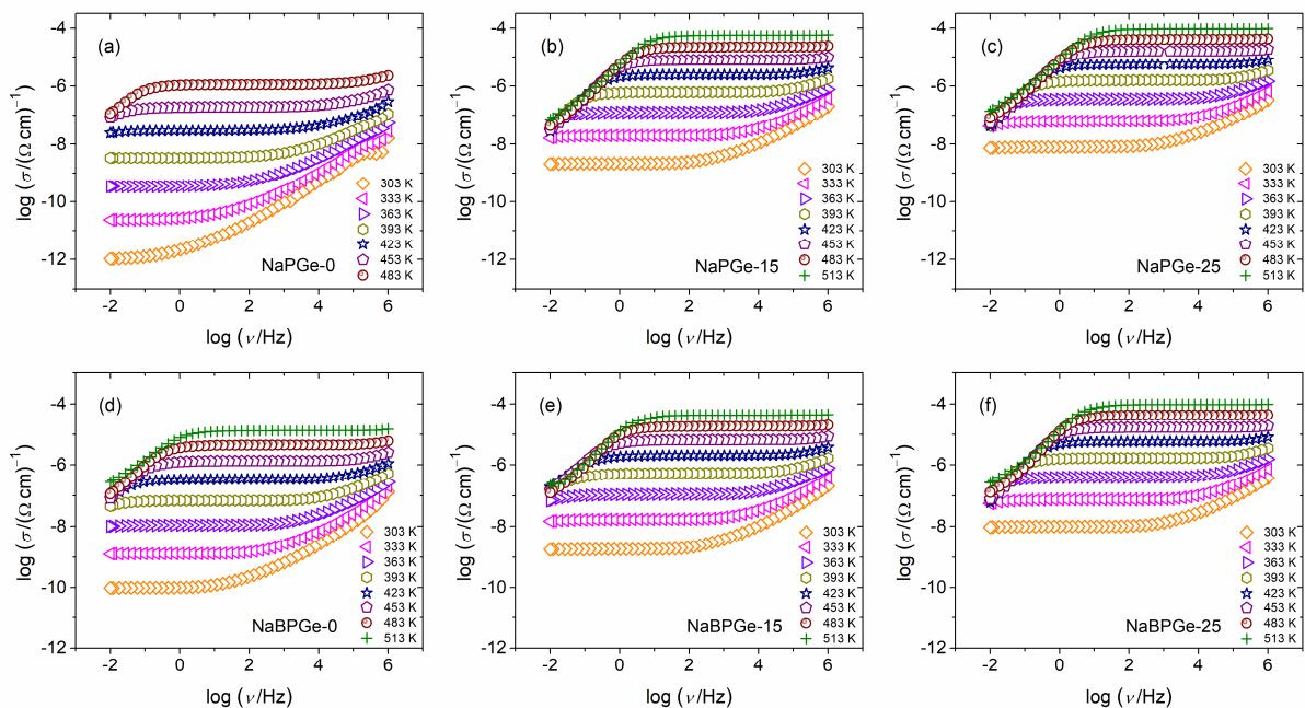
Slika 74. Spektri provodnosti za odabrana stakla ( $x = 0, 15 \text{ i } 25 \text{ mol}\%$ ) iz serija C:  $40\text{Na}_2\text{O}-(60-x)\text{P}_2\text{O}_5-x\text{GeO}_2$  (a-c) i D:  $40\text{Na}_2\text{O}-10\text{B}_2\text{O}_3-(50-x)\text{P}_2\text{O}_5-x\text{GeO}_2$  (d-f).
