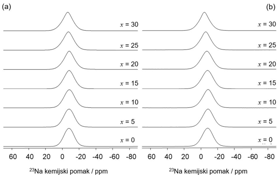
Slika 51.  $^{23}\text{Na}$  MAS NMR spektri snimljeni na 18,8 T za stakla iz serije C:  $40\text{Na}_2\text{O}-(60-x)\text{P}_2\text{O}_5-x\text{GeO}_2$  (a) i serije D:  $40\text{Na}_2\text{O}-10\text{B}_2\text{O}_3-(50-x)\text{P}_2\text{O}_5-x\text{GeO}_2$  (b).
