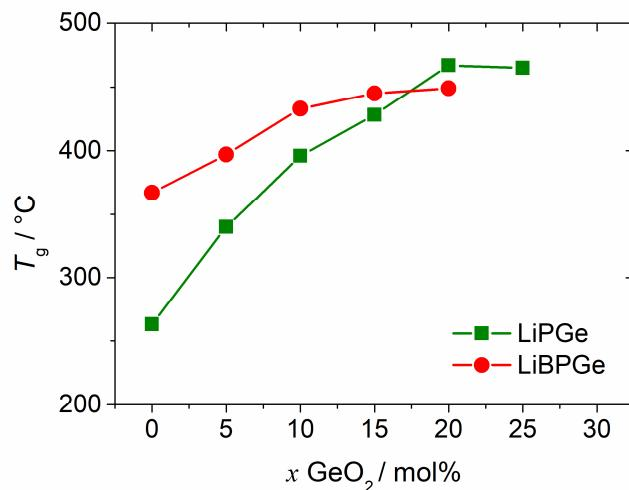
Slika 29. Ovisnost  $T_g$  o udjelu  $\text{GeO}_2$  za serije A:  $40\text{Li}_2\text{O}-(60-x)\text{P}_2\text{O}_5-x\text{GeO}_2$  i B:  $40\text{Li}_2\text{O}-10\text{B}_2\text{O}_3-(50-x)\text{P}_2\text{O}_5-x\text{GeO}_2$ .
