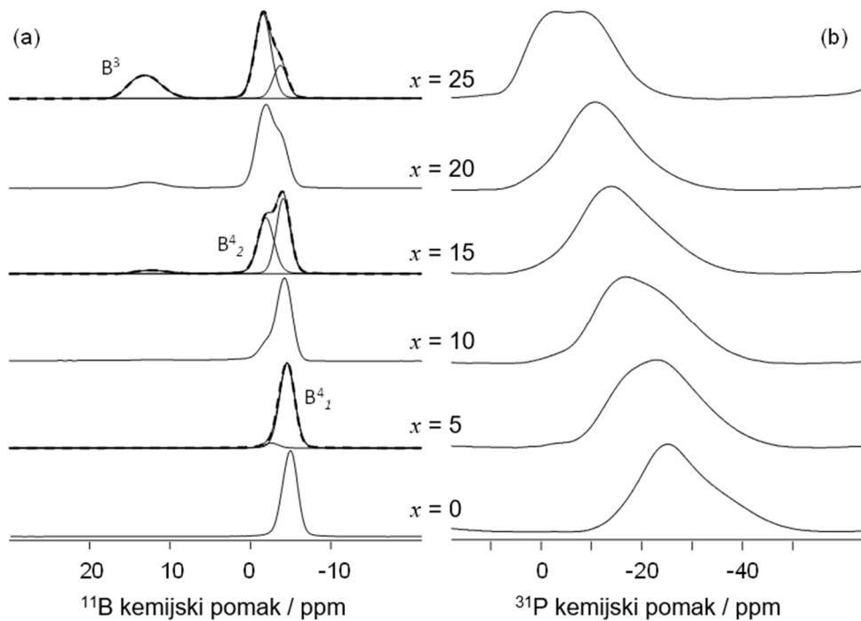
Slika 38.  $^{11}\text{B}$  (a) i  $^{31}\text{P}$  MAS NMR spektri (b) za stakla iz serije B:  $40\text{Li}_2\text{O}-10\text{B}_2\text{O}_3-(50-x)\text{P}_2\text{O}_5-x\text{GeO}_2$ .
