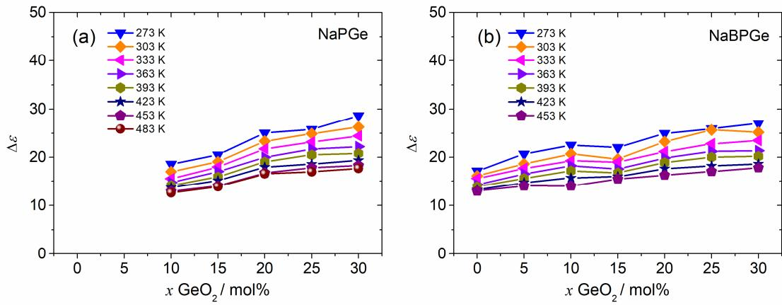
Slika 79. Trendovi ovisnosti  $\Delta\epsilon$  o udjelu  $\text{GeO}_2$  za natrijeve serije stakala C:  $40\text{Na}_2\text{O}-(60-x)\text{P}_2\text{O}_5-x\text{GeO}_2$  (a) i D:  $40\text{Na}_2\text{O}-10\text{B}_2\text{O}_3-(50-x)\text{P}_2\text{O}_5-x\text{GeO}_2$  (b).
