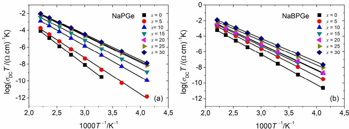
Slika 76. Ovisnost  $\log(\sigma_{DC}T)$  o recipročnoj temperaturi,  $1/T$ , za stakla iz serija C:  $40\text{Na}_2\text{O}-(60-x)\text{P}_2\text{O}_5-x\text{GeO}_2$  (a) i D:  $40\text{Na}_2\text{O}-10\text{B}_2\text{O}_3-(50-x)\text{P}_2\text{O}_5-x\text{GeO}_2$  (b).
