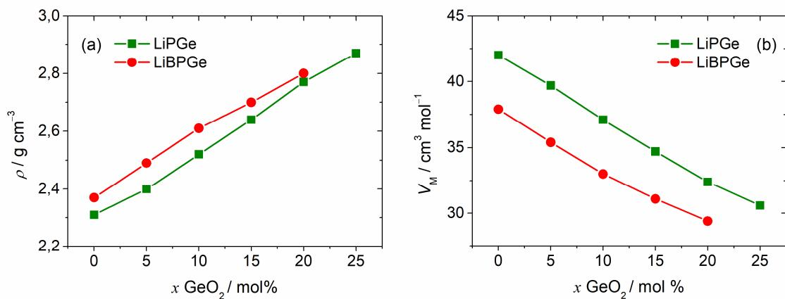
Slika 27. Ovisnost gustoće,  $\rho$ , (a) i molarnog volumena,  $V_M$ , (b) o udjelu dodanog  $\text{GeO}_2$  za stakla iz serija A:  $40\text{Li}_2\text{O}-(60-x)\text{P}_2\text{O}_5-x\text{GeO}_2$  i B:  $40\text{Li}_2\text{O}-10\text{B}_2\text{O}_3-(50-x)\text{P}_2\text{O}_5-x\text{GeO}_2$ .
