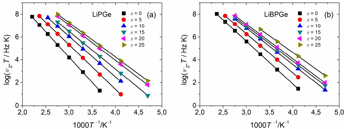
Slika 63. Ovisnost  $\log(\nu_{Z''}T)$  o recipročnoj temperaturi,  $1/T$ , za stakla iz serija A:  $40\text{Li}_2\text{O}-(60-x)\text{P}_2\text{O}_5-x\text{GeO}_2$  (a) i B:  $40\text{Li}_2\text{O}-10\text{B}_2\text{O}_3-(50-x)\text{P}_2\text{O}_5-x\text{GeO}_2$  (b).
