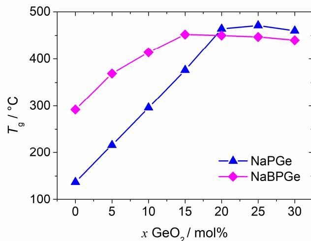
Slika 31. Ovisnosti  $T_g$  o udjelu GeO<sub>2</sub> za serije C: 40Na<sub>2</sub>O-(60- $x$ )P<sub>2</sub>O<sub>5</sub>- $x$ GeO<sub>2</sub> i D: 40Na<sub>2</sub>O-10B<sub>2</sub>O<sub>3</sub>-(50- $x$ )P<sub>2</sub>O<sub>5</sub>- $x$ GeO<sub>2</sub>.
