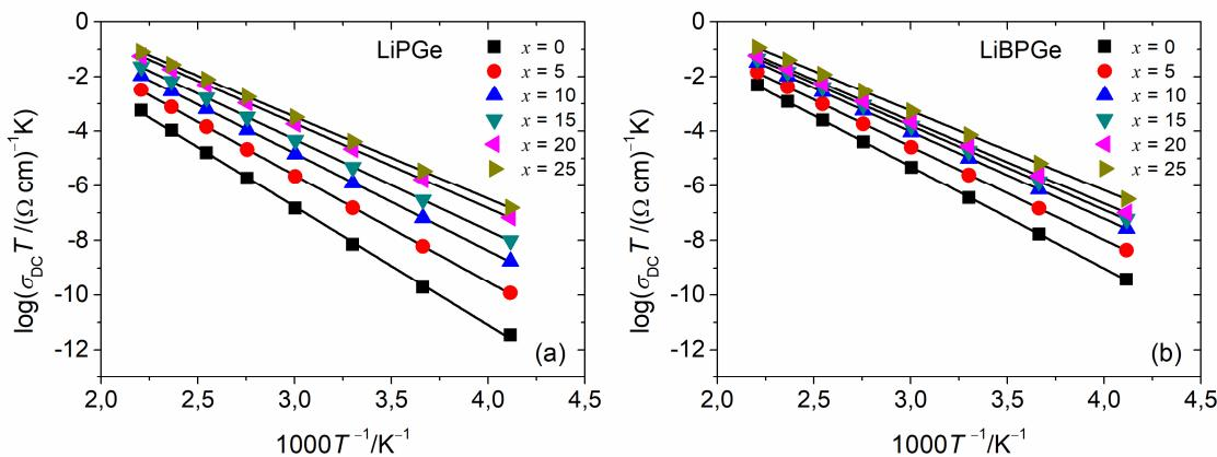
Slika 56. Ovisnost  $\log(\sigma_{DC}T)$  o recipročnoj temperaturi,  $1/T$ , za stakla iz serija A:  $40\text{Li}_2\text{O}-(60-x)\text{P}_2\text{O}_5-x\text{GeO}_2$  (a) i B:  $40\text{Li}_2\text{O}-10\text{B}_2\text{O}_3-(50-x)\text{P}_2\text{O}_5-x\text{GeO}_2$  (b).
