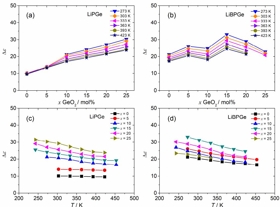
Slika 59. Trendovi ovisnosti  $\Delta\epsilon$  o udjelu  $\text{GeO}_2$  (a-b) te o temperaturi mjerena (c-d) za serije stakala A:  $40\text{Li}_2\text{O}-(60-x)\text{P}_2\text{O}_5-x\text{GeO}_2$  i B:  $40\text{Li}_2\text{O}-10\text{B}_2\text{O}_3-(50-x)\text{P}_2\text{O}_5-x\text{GeO}_2$ .
