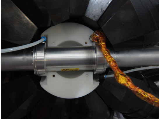
FIG. 3. Picture of the fission chamber placed in the center of the TAC. In white, half of the borated polyethylene neutron absorber shell.
