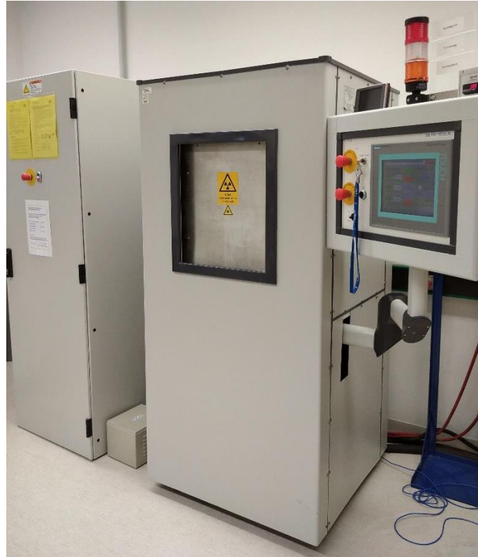
Figure 2.15. The radiation machine (Gulmay) used to irradiate MS2 phage with X-rays.
