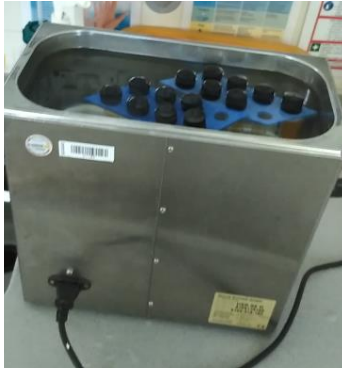
Figure 2.7. Tubes with soft agar cooling down at 48 °C after melting and before adding bacteria inside.
