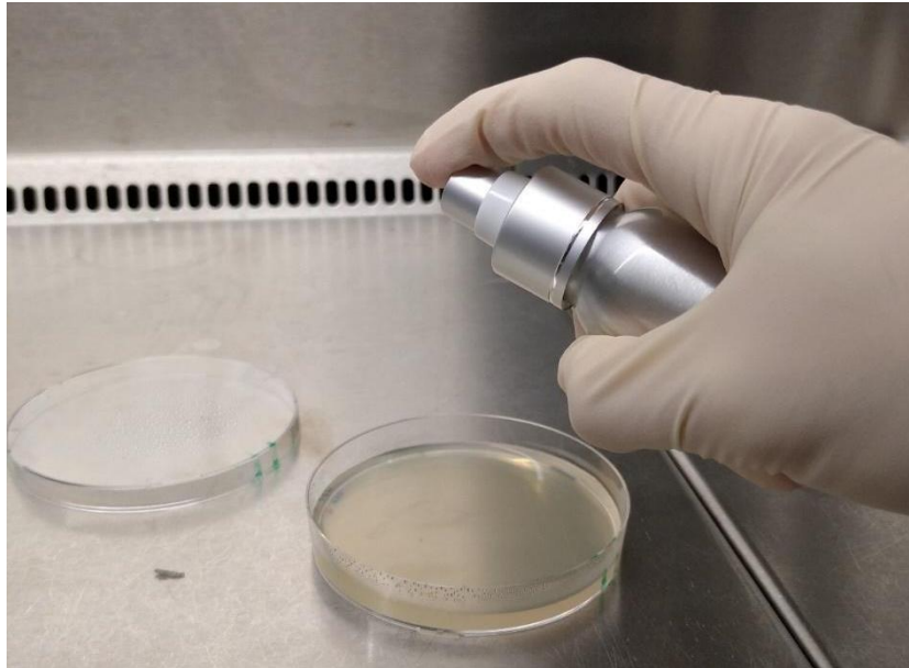
Figure 2.17. Applying a positive control for testing of MS2 phage transmission in aerosols. The phages ( 4.18 \times 10^7 \pm 1.61 \times 10^7 PFU/mL) were sprayed onto the fresh bacterial lawn at \sim 10 cm distance.
