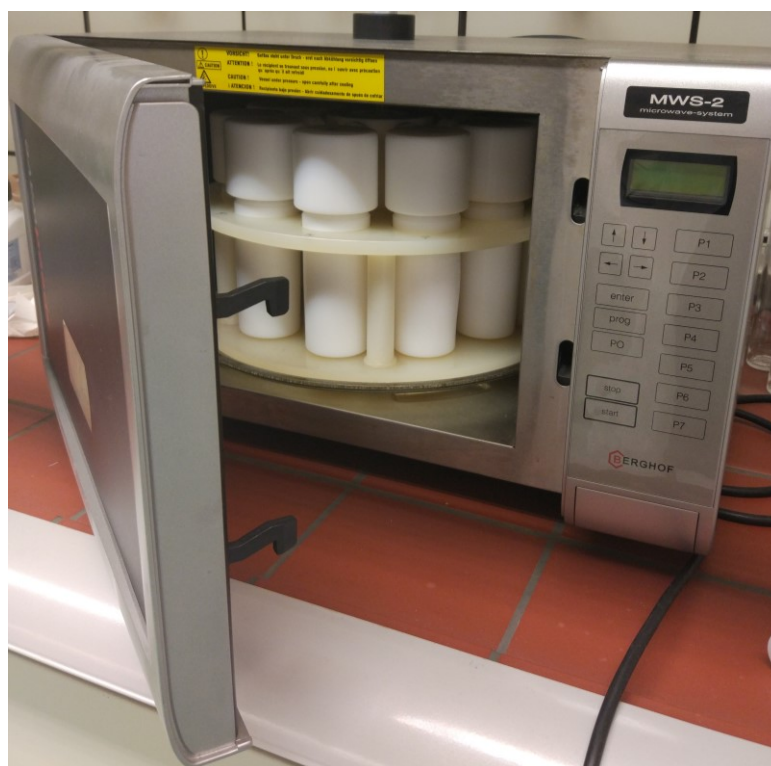
Slika 12. Uređaj MWS-2 Microwave System Speedweve Berghof
