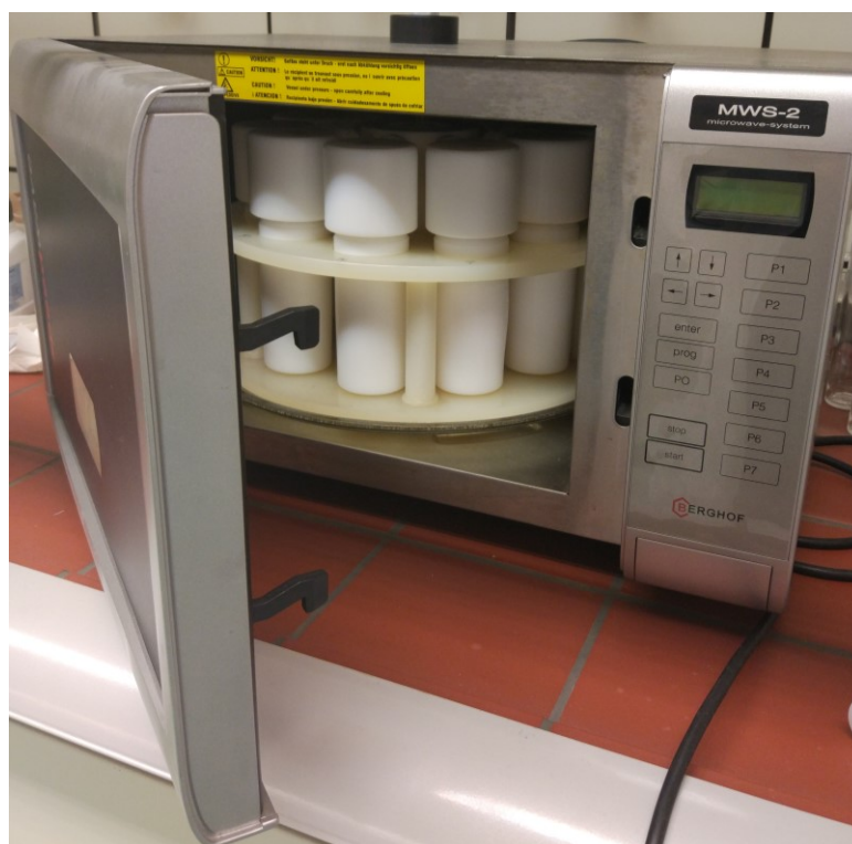
Slika 12. Uređaj MWS-2 Microwave System Speedweve Berghof
