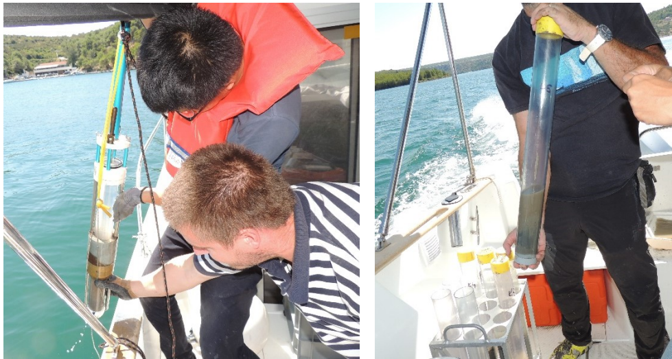
Figure 4.2. Sediment sampling using Uwitec gravity corer
