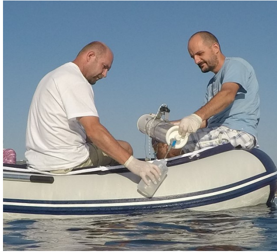
Figure 4.3. Filling 1 L FEP bottle with the sample taken with the horizontal water sampler
