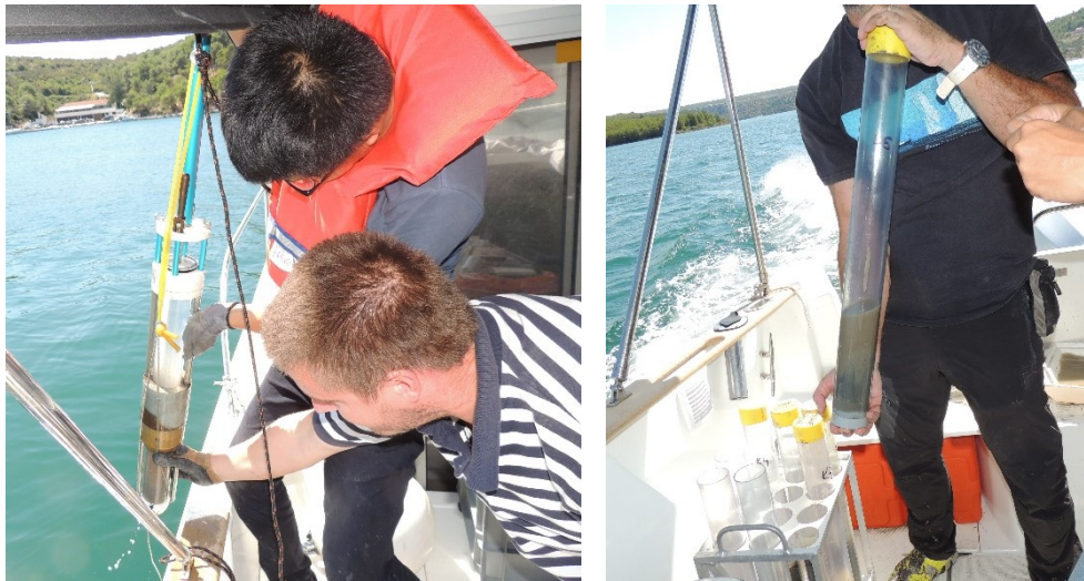
Figure 4.2. Sediment sampling using Uwitec gravity corer
