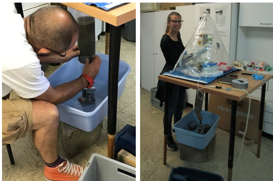
Figure 4.5. Positioning of the hydraulic jack below the sediment core previously installed on the slicing table (left) and working in pyramidal glove box (right)
