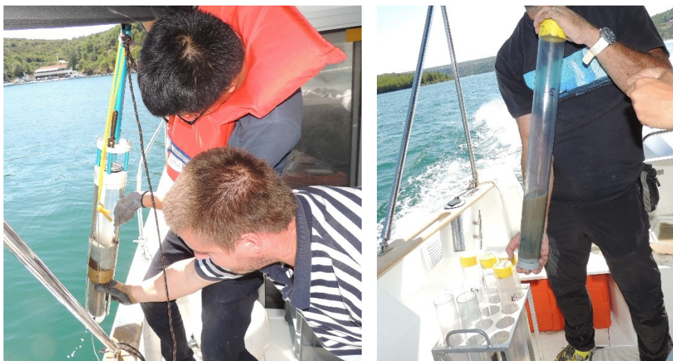
Figure 4.2. Sediment sampling using Uwitec gravity corer
