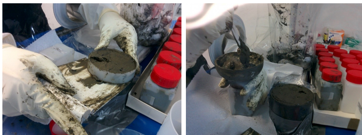
Figure 4.6. Slicing the sediment core under the inert atmosphere (left) and transferring the obtained slice into HDPE container through the funnel (right)
