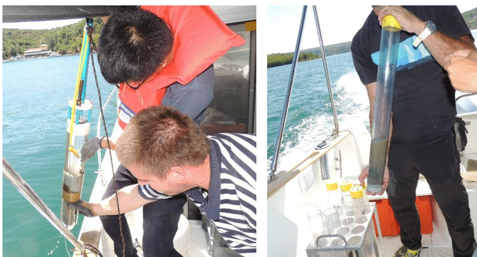
Figure 4.2. Sediment sampling using Uwitec gravity corer
