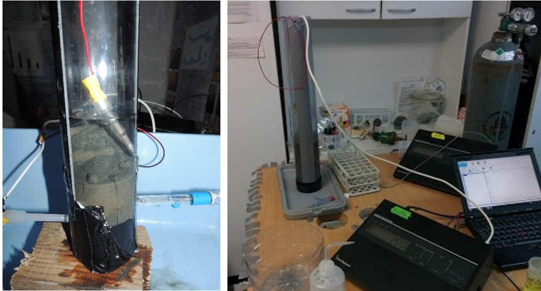
Figure 4.10. Measuring of the pH and Eh in the sediment pore water by using combination of electrodes and an expandable ion analyzer EA 920 (Orion Research)
