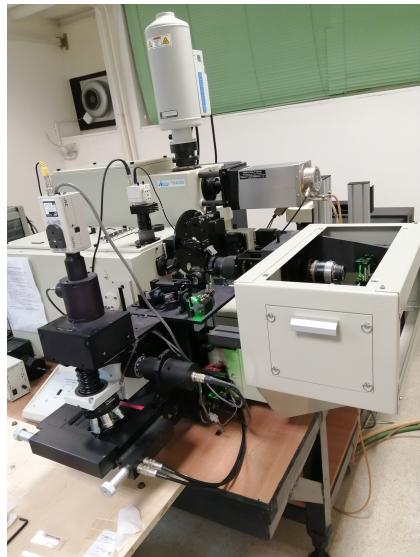
Slika 2.18: Ramanov spektrometar HORIBA Jobin Yvon model T64000
