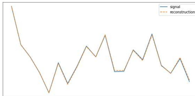
Figure 2.8: A synthetic signal vector (blue, solid) approximated by a 5-sparse coefficient vector using a 20 \times 50 dictionary (the approximation is orange and dashed)
